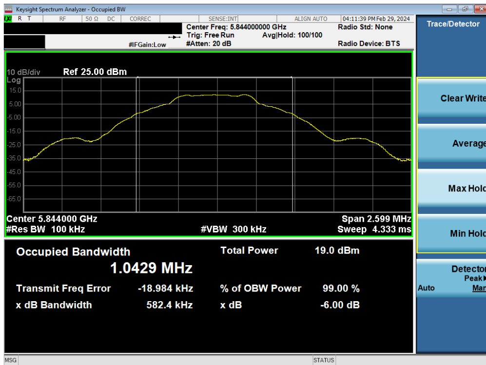
Plot 7-12. 6dB BW & 99% OBW Antenna WF7a (BDR GFSK, ePA 5844MHz)
