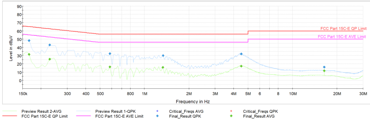
Plot 7-720. AC Line Conducted Plot with CDD 11ax - SU Ch.6 (L1, with AC/DC Adapter)
