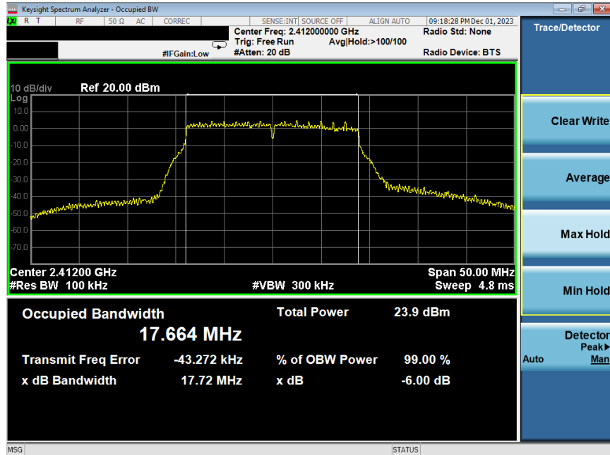
Plot 7-43. 6 dB BW and 99% OBW Plot Antenna WF7b (802.11n (2.4GHz) – Ch. 1) – MCS4
