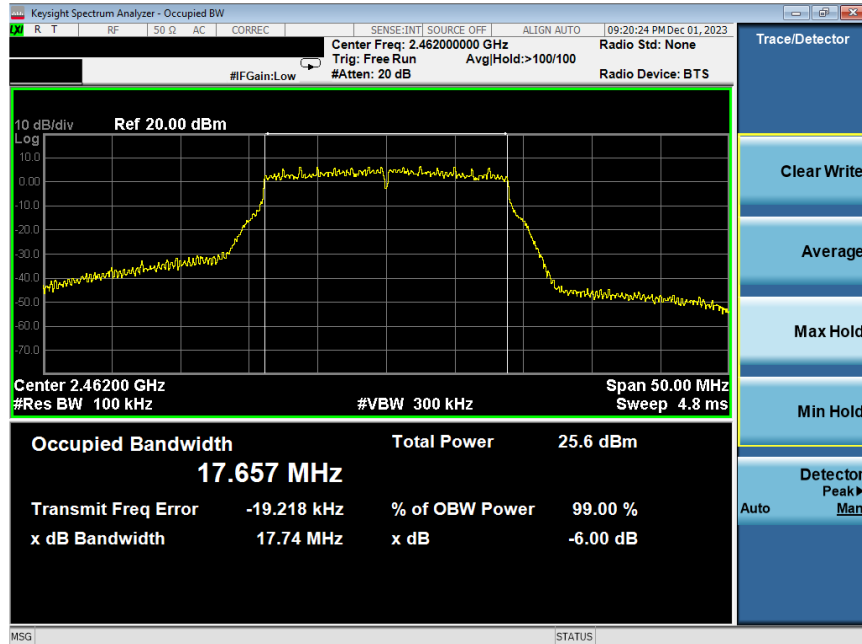
Plot 7-45. 6 dB BW and 99% OBW Plot Antenna WF7b (802.11n (2.4GHz) – Ch. 11) – MCS4
