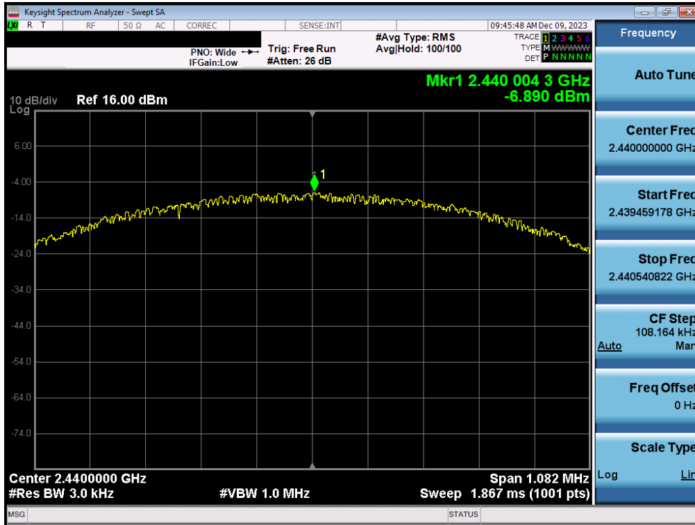
Plot 7-45. Power Spectral Density Plot Antenna WF8 (Bluetooth (LE), 1Mbps, iPA – Ch. 19)
