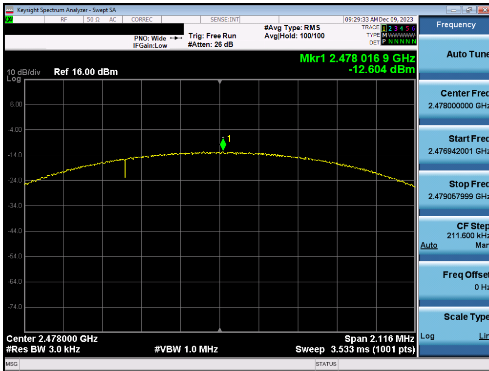
Plot 7-60. Power Spectral Density Plot Antenna WF7b (Bluetooth (LE), 2Mbps, iPA – Ch. 38)
