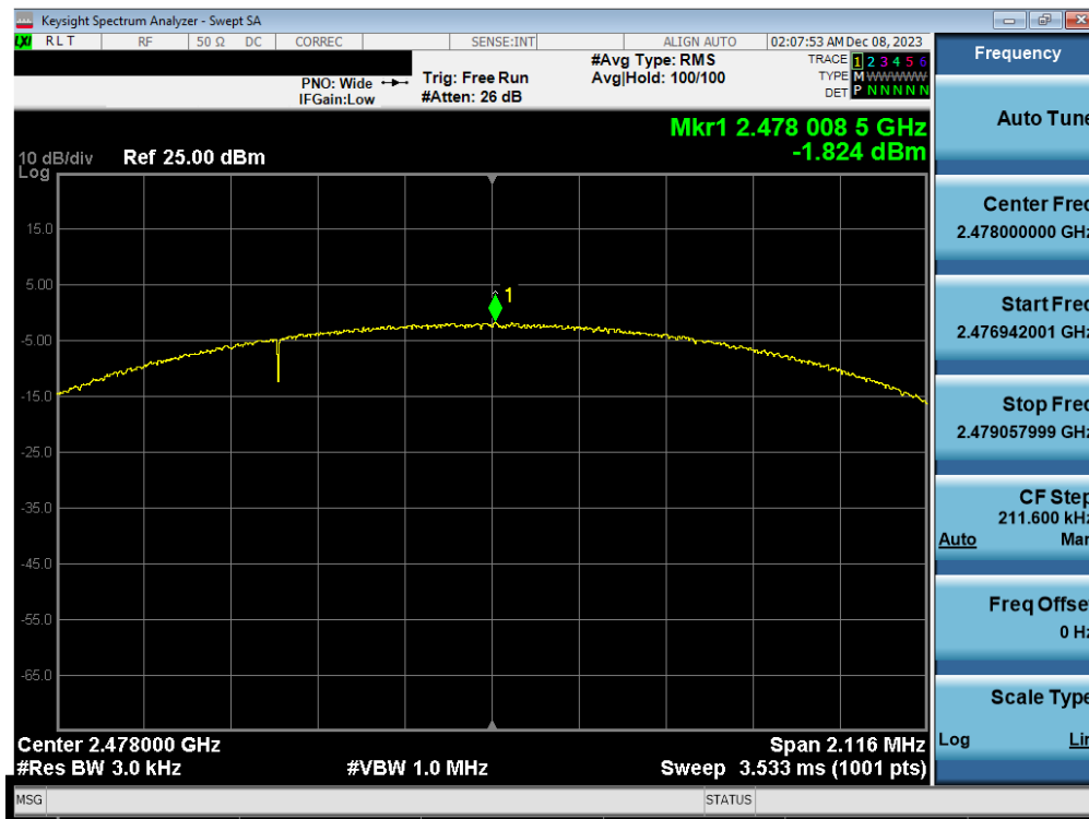
Plot 7-54. Power Spectral Density Plot Antenna WF7b (Bluetooth (LE), 2Mbps, ePA – Ch. 38)
