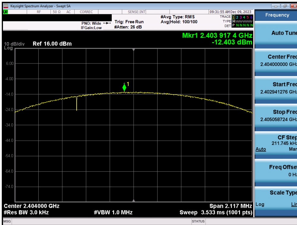
Plot 7-34. Power Spectral Density Plot Antenna WF7b (Bluetooth (LE), 2Mbps, iPA – Ch. 1)
