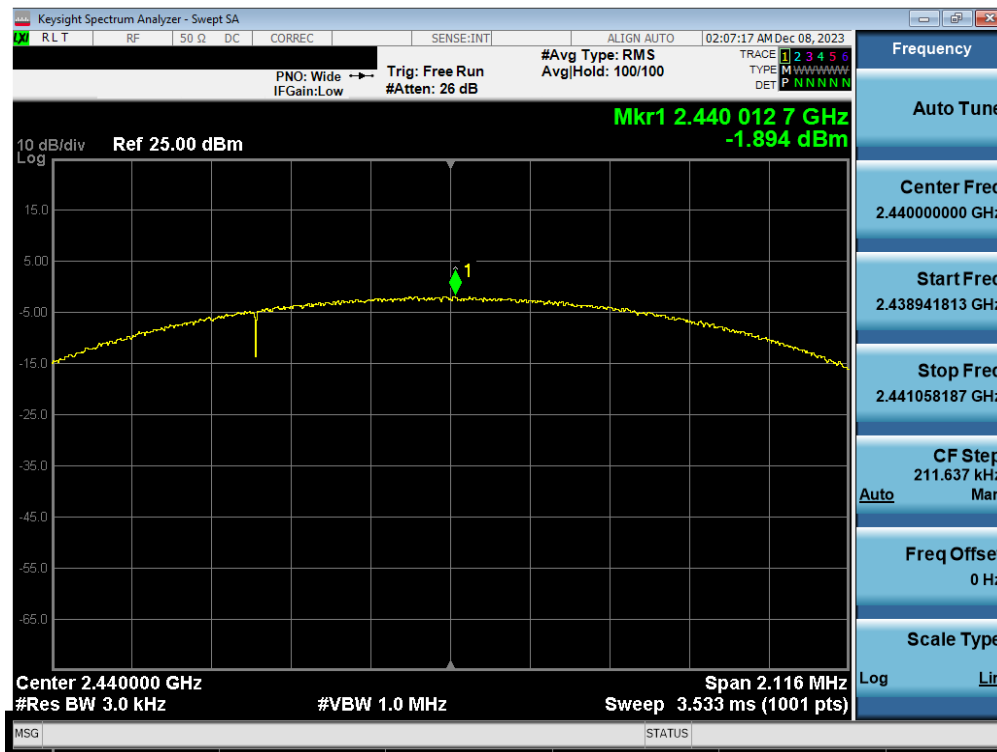
Plot 7-52. Power Spectral Density Plot Antenna WF7b (Bluetooth (LE), 2Mbps, ePA – Ch. 19)
