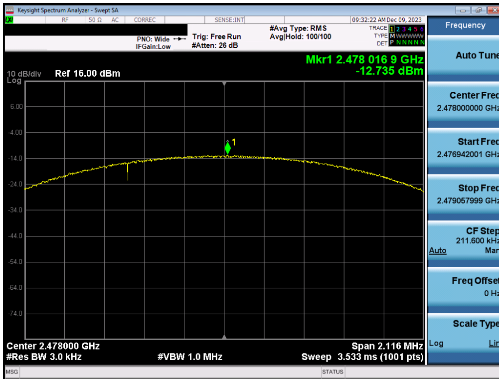
Plot 7-36. Power Spectral Density Plot Antenna WF7b (Bluetooth (LE), 2Mbps, iPA – Ch. 38)
