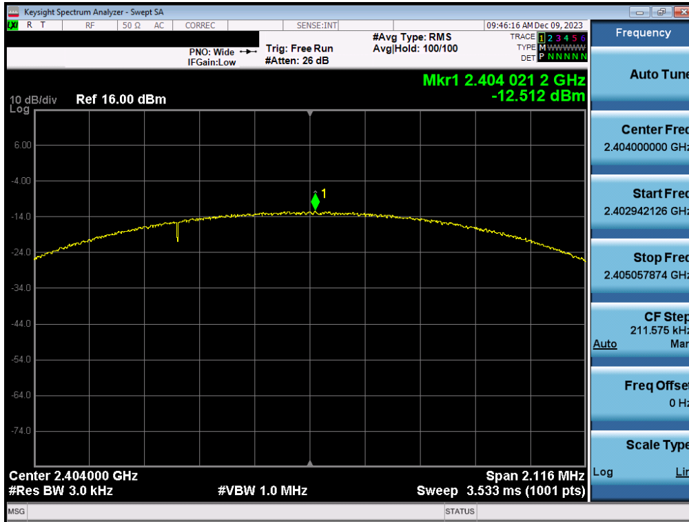
Plot 7-55. Power Spectral Density Plot Antenna WF8 (Bluetooth (LE), 2Mbps, iPA – Ch. 1)
