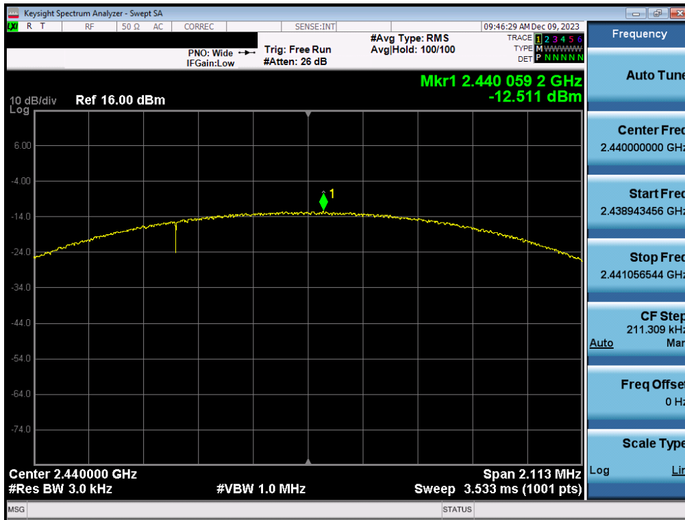
Plot 7-57. Power Spectral Density Plot Antenna WF8 (Bluetooth (LE), 2Mbps, iPA – Ch. 19)
