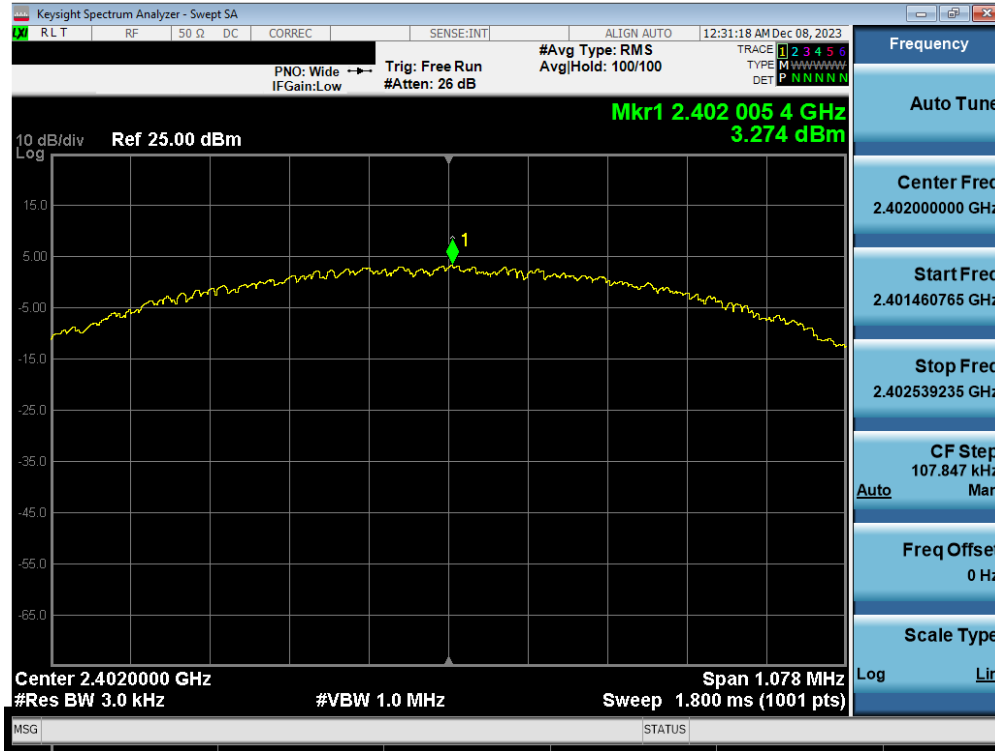
Plot 7-37. Power Spectral Density Plot Antenna WF8 (Bluetooth (LE), 1Mbps, ePA – Ch. 0)
