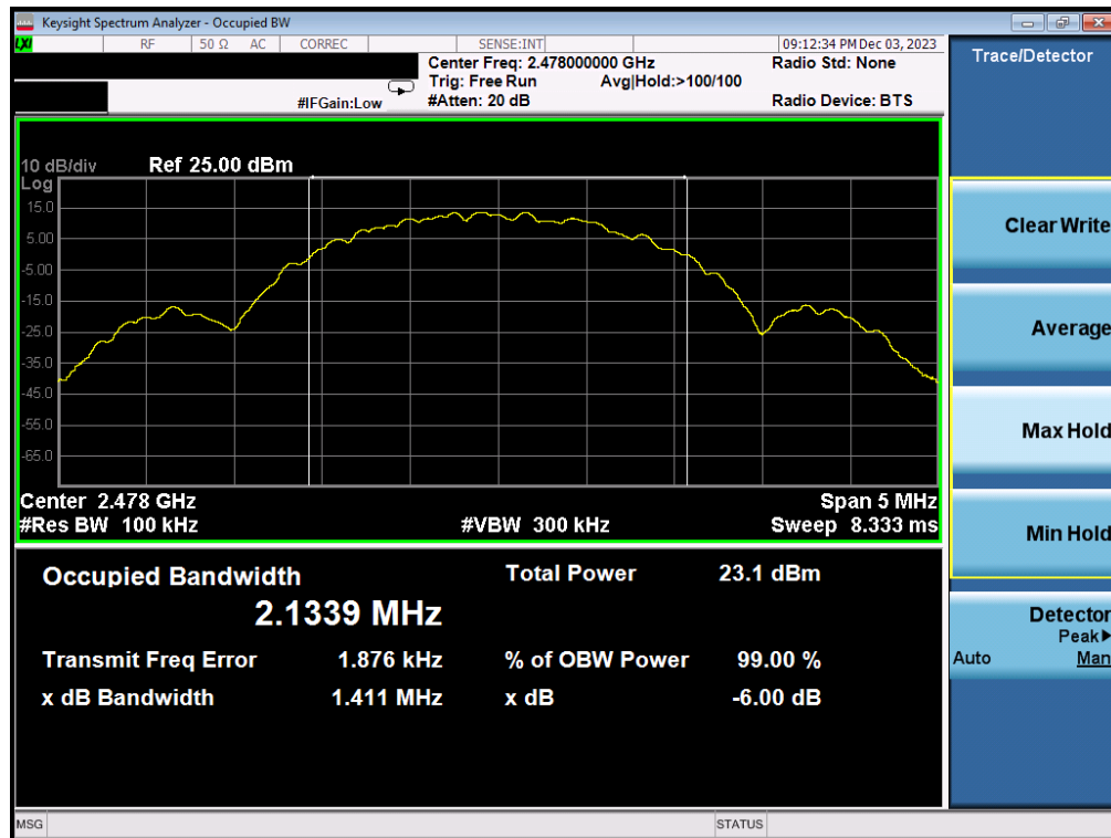
Plot 7-12. 6dB BW & 99% OBW Plot Antenna WF7b (Bluetooth (LE), 2Mbps, ePA – Ch. 38)
