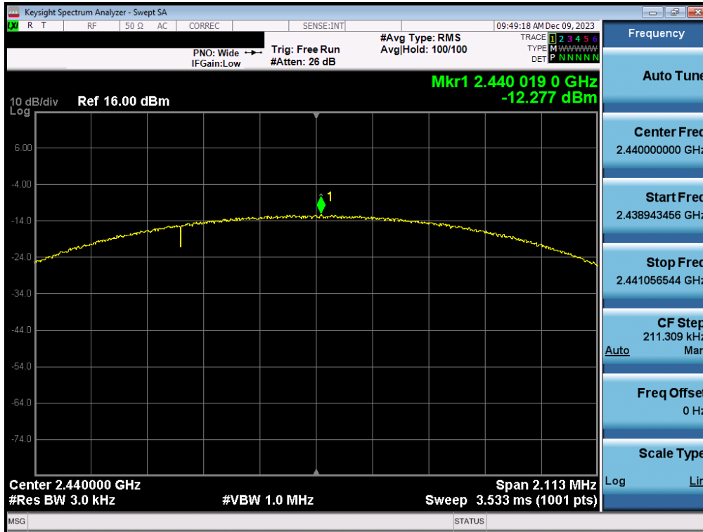
Plot 7-23. Power Spectral Density Plot Antenna WF8 (Bluetooth (LE), 2Mbps, iPA – Ch. 19)
