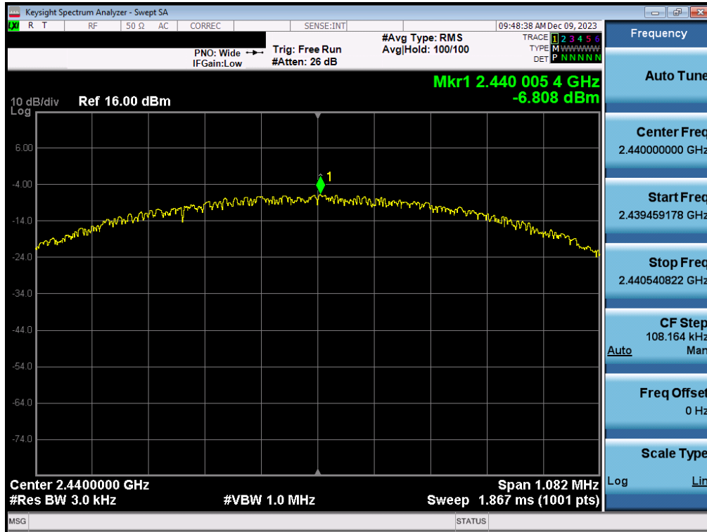
Plot 7-17. Power Spectral Density Plot Antenna WF8 (Bluetooth (LE), 1Mbps, iPA – Ch. 19)
