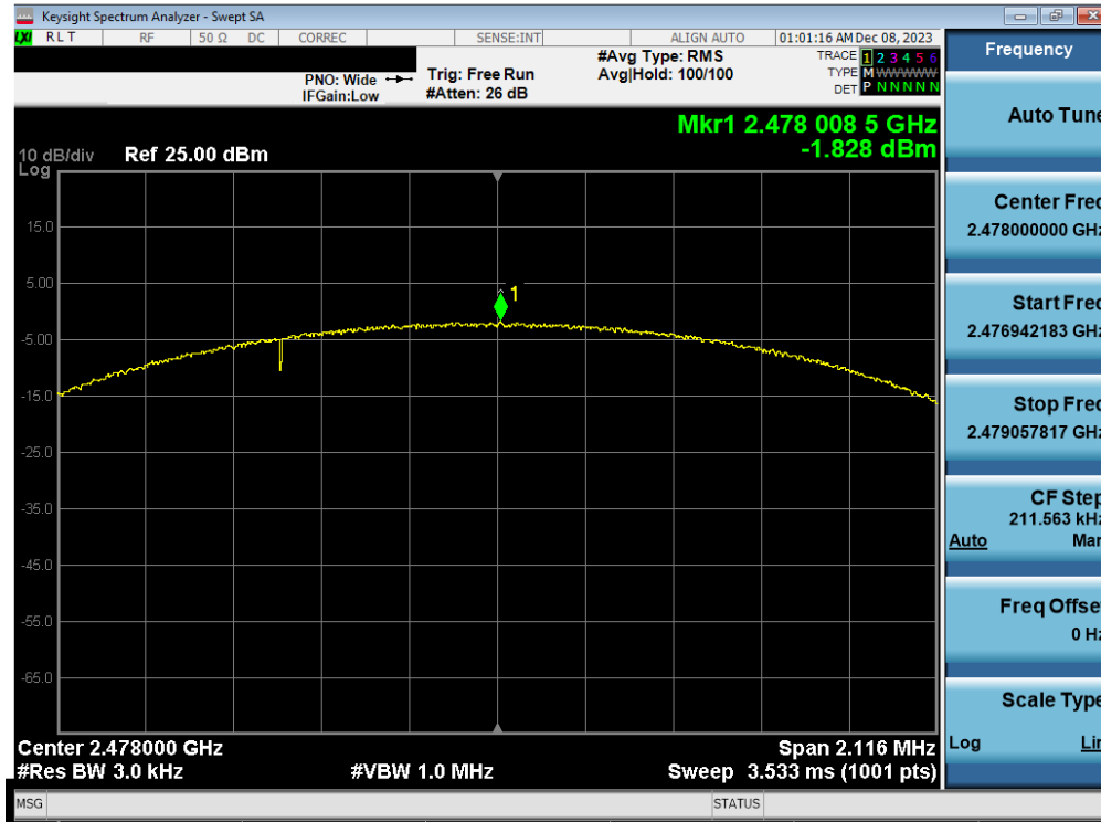
Plot 7-53. Power Spectral Density Plot Antenna WF8 (Bluetooth (LE), 2Mbps, ePA – Ch. 38)
