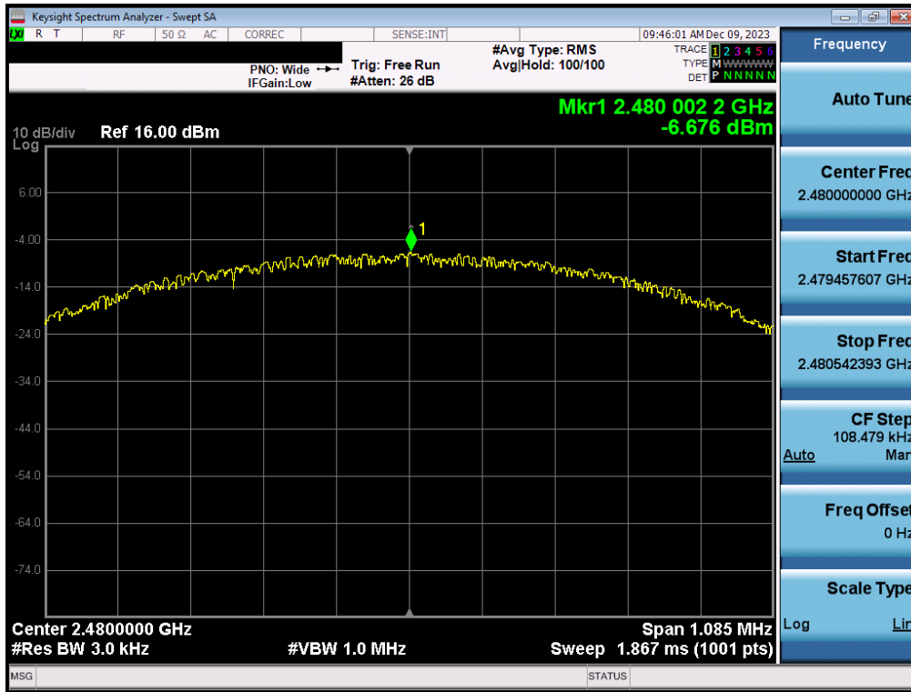
Plot 7-47. Power Spectral Density Plot Antenna WF8 (Bluetooth (LE), 1Mbps, iPA – Ch. 39)
