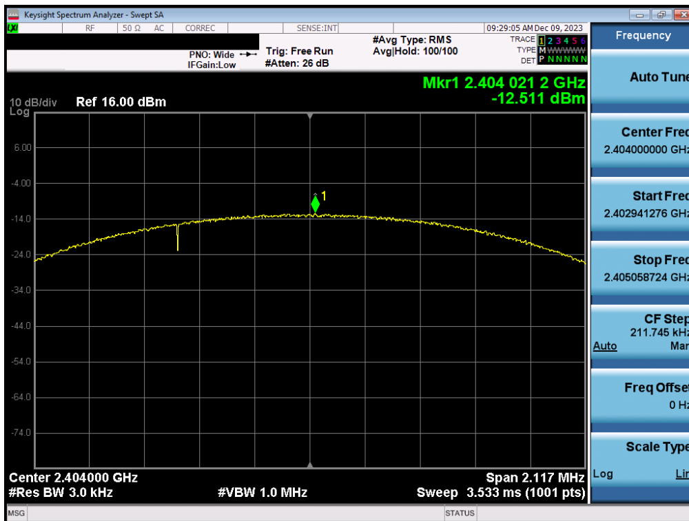
Plot 7-56. Power Spectral Density Plot Antenna WF7b (Bluetooth (LE), 2Mbps, iPA – Ch. 1)
