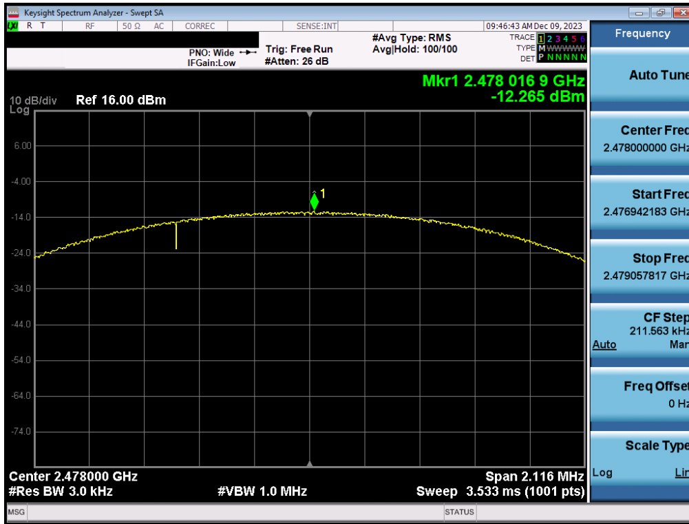
Plot 7-59. Power Spectral Density Plot Antenna WF8 (Bluetooth (LE), 2Mbps, iPA – Ch. 38)
