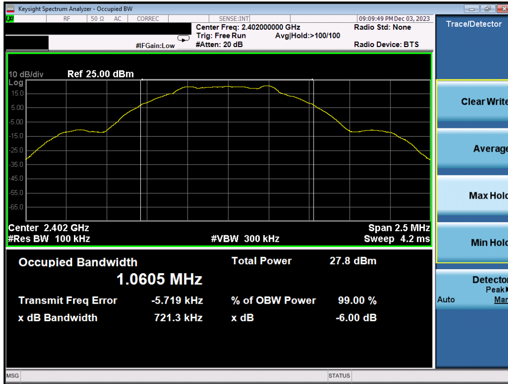
Plot 7-7. 6dB BW & 99% OBW Plot Antenna WF7b (Bluetooth (LE), 1Mbps, ePA – Ch. 0)
