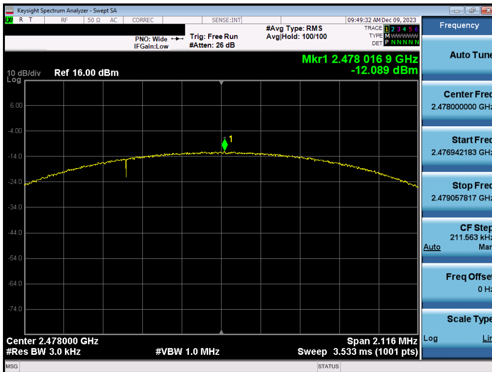
Plot 7-24. Power Spectral Density Plot Antenna WF8 (Bluetooth (LE), 2Mbps, iPA – Ch. 38)
