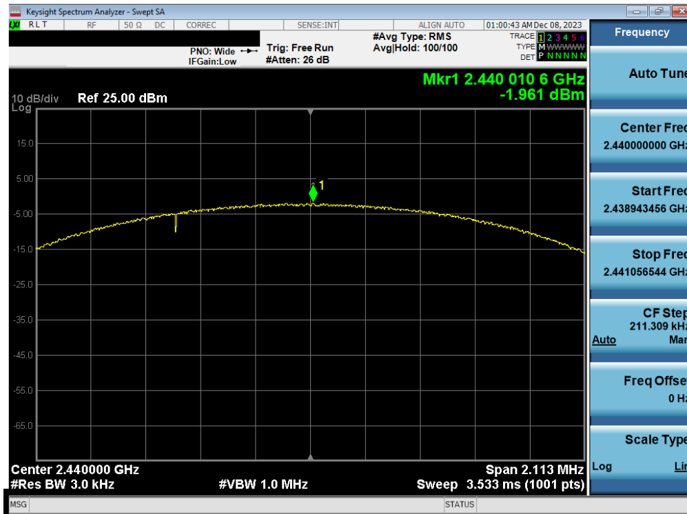
Plot 7-51. Power Spectral Density Plot Antenna WF8 (Bluetooth (LE), 2Mbps, ePA – Ch. 19)
