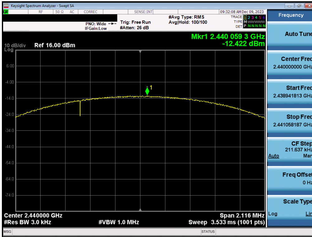
Plot 7-35. Power Spectral Density Plot Antenna WF7b (Bluetooth (LE), 2Mbps, iPA – Ch. 19)
