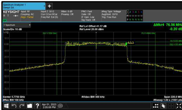
Figure 202 - 802.11ax HE80 SU Minimum 6 dB EBW
