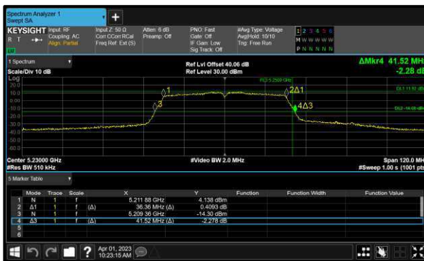
Figure 234 - 802.11n HT40 Minimum 99% OBW
