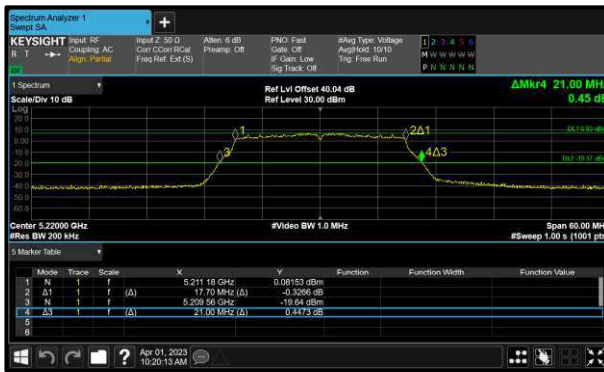
Figure 232 - 802.11n HT20 Minimum 99% OBW
