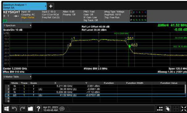
Figure 178 - 802.11n HT40 Minimum 99% OBW
