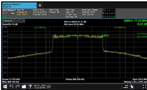
Figure 172 - 802.11ax HE80 SU Minimum 6 dB EBW
