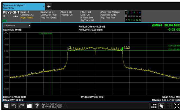
Figure 170 - 802.11ax HE40 SU Minimum 6 dB EBW
