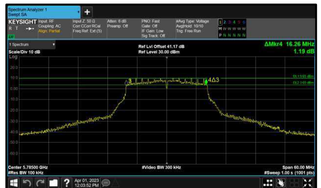
Figure 161 - 802.11a Maximum 6 dB EBW
