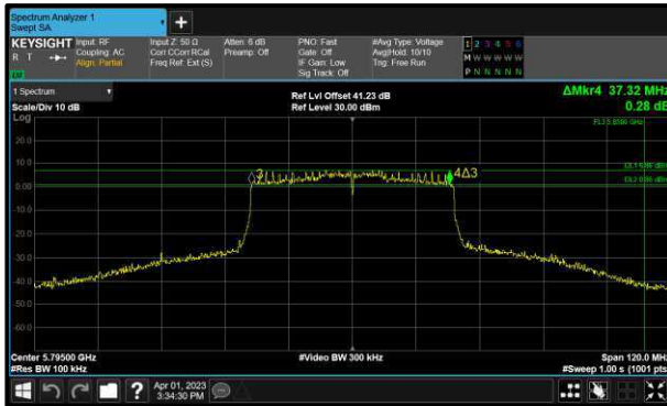
Figure 228 - 802.11ax HE40 SU Minimum 6 dB EBW
