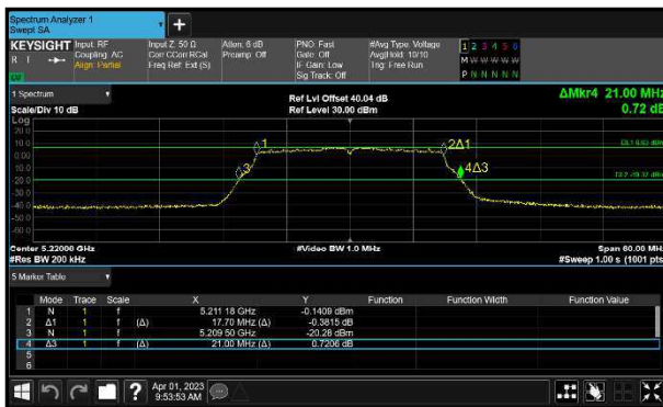
Figure 204 - 802.11n HT20 Minimum 99% OBW
