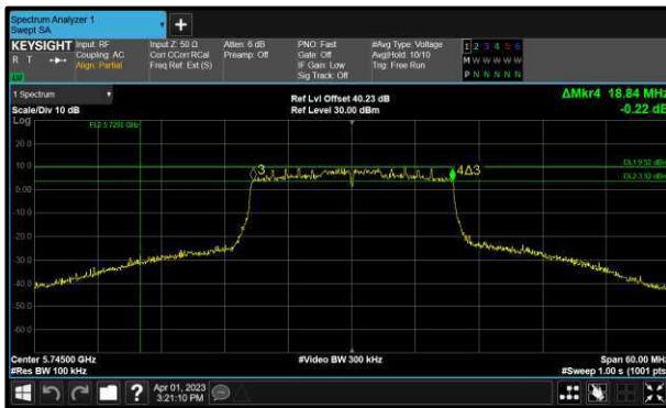
Figure 226 - 802.11ax HE20 SU Minimum 6 dB EBW
