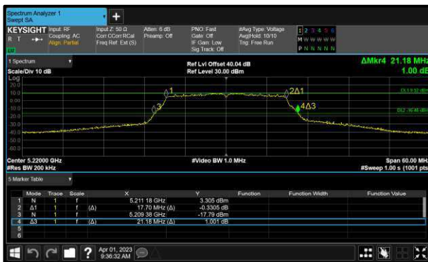
Figure 176 - 802.11n HT20 Minimum 99% OBW
