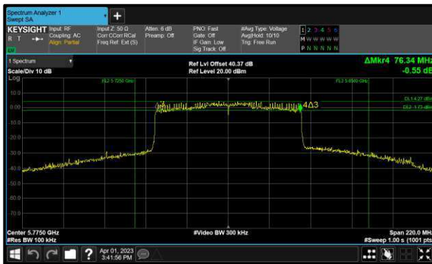
Figure 230 - 802.11ax HE80 SU Minimum 6 dB EBW
