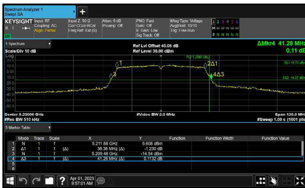
Figure 206 - 802.11n HT40 Minimum 99% OBW
