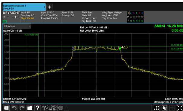
Figure 160 - 802.11a Minimum 6 dB EBW
