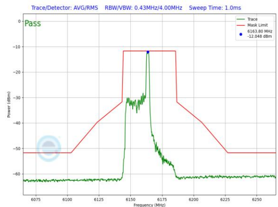
Plot 7-1420. LPI In-Band Emission Plot SDM Diversity Antenna 1b (40MHz 802.11ax RU26 (UNII Band 5) – Ch. 43)
