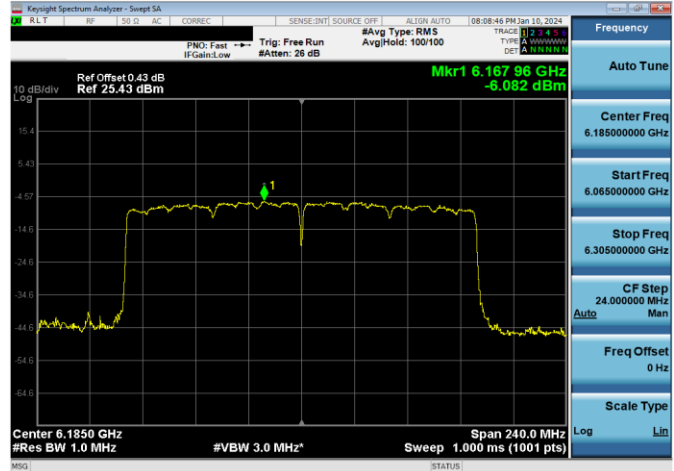
Plot 7-560. LPI Power Spectral Density Plot Antenna 1b (160MHz 802.11ax RU996x2 (UNII Band 5) – Ch. 47)
