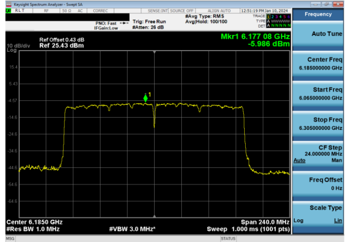
Plot 7-496. LPI Power Spectral Density Plot Antenna 3b (160MHz 802.11ax RU996x2 (UNII Band 5) – Ch. 47)
