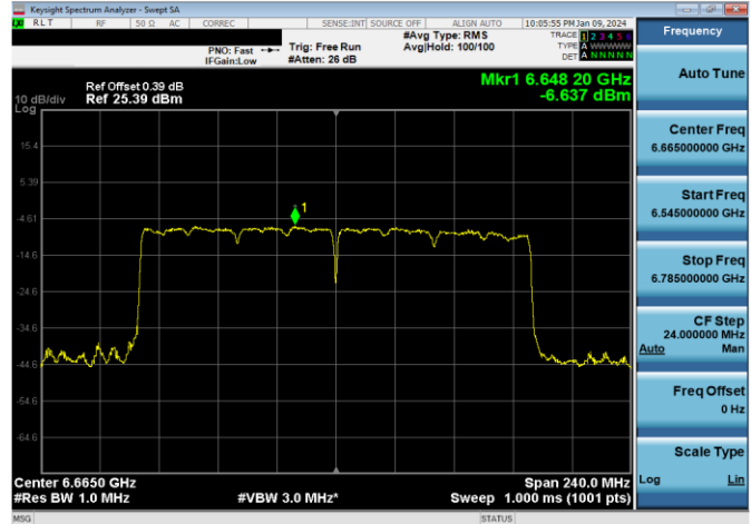
Plot 7-416. SP Power Spectral Density Plot CDD Diversity Antenna 1b (160MHz 802.11ax RU996x2 (UNII Band 7) – Ch. 143)
