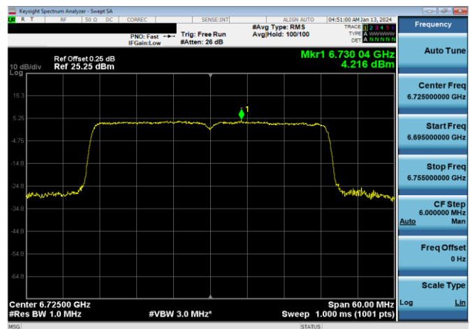
Plot 7-336. SP Power Spectral Density Plot CDD Primary Antenna 3b (40MHz 802.11ax RU484 (UNII Band 7) – Ch. 155)
