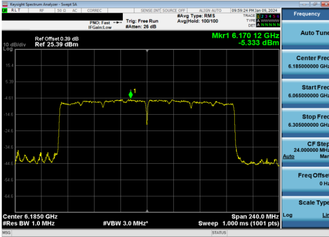
Plot 7-384. SP Power Spectral Density Plot CDD Diversity Antenna 1b (160MHz 802.11ax RU996x2 (UNII Band 5) – Ch. 47)
