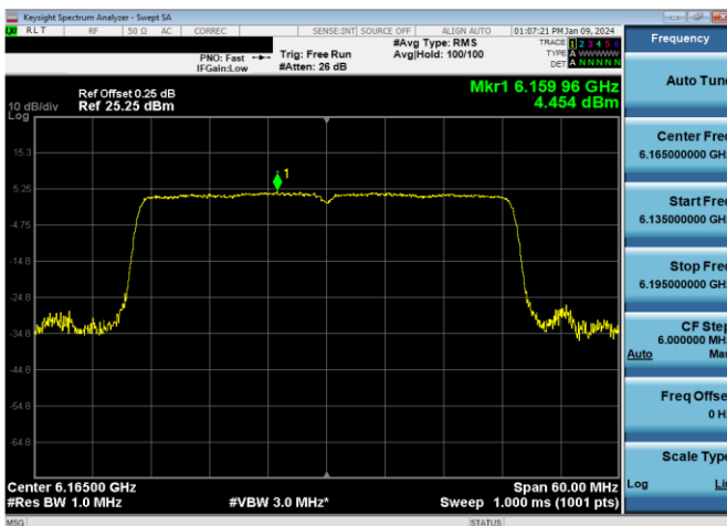
Plot 7-303. SP Power Spectral Density Plot CDD Primary Antenna 5T (40MHz 802.11ax RU484 (UNII Band 5) - Ch. 43)
