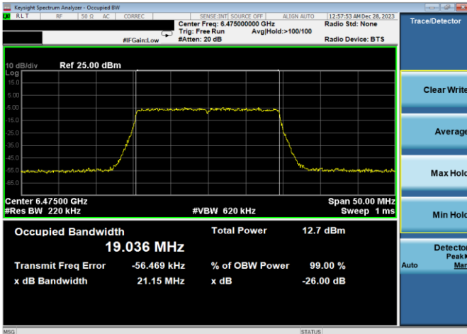
Plot 7-20. 26dB & 99% Bandwidth Plot Antenna 5T (20MHz 802.11ax RU242 (UNII Band 6) – Ch. 105)
