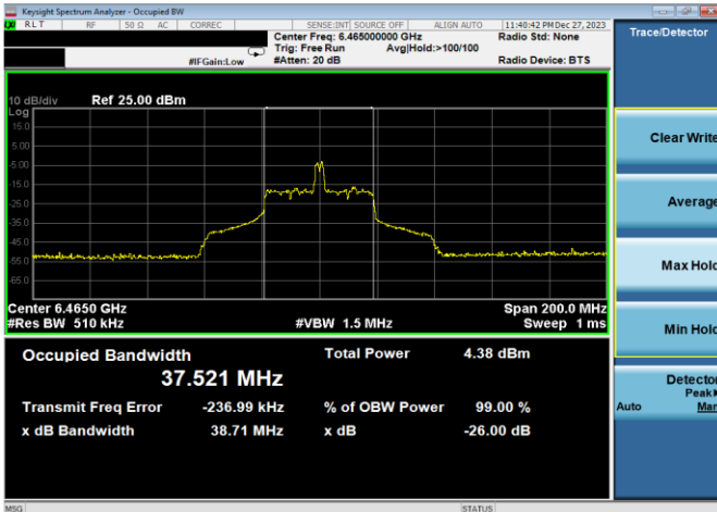
Plot 7-26. 26dB & 99% Bandwidth Plot Antenna 5T (80MHz 802.11ax RU26 (UNII Band 6) – Ch. 103)
