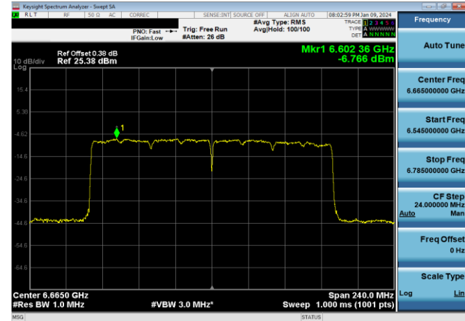
Plot 7-738. Power Spectral Density Plot CDD Diversity Antenna 1b Standard Power (160MHz 802.11ax (UNII Band 7) – Ch. 143, MCS11)
