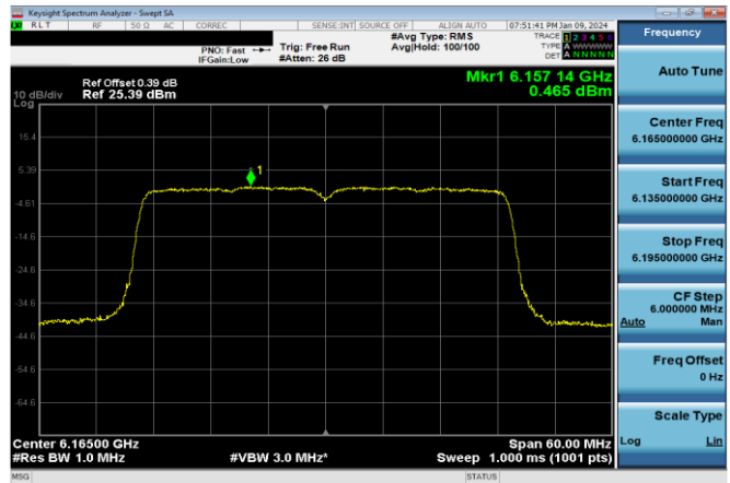
Plot 7-726. Power Spectral Density Plot CDD Diversity Antenna 1b Standard Power (40MHz 802.11ax (UNII Band 5) – Ch. 43, MCS11)
