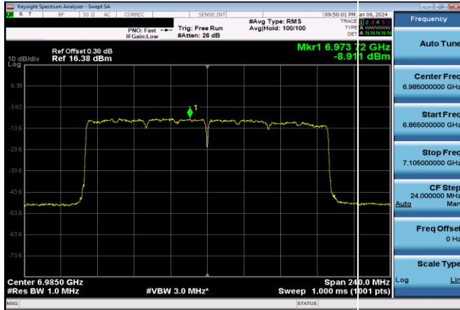
Plot 7-689. Power Spectral Density Plot SDM Diversity Antenna 3b LPI (160MHz 802.11ax (UNII Band 8) – Ch. 207, MCS11)
