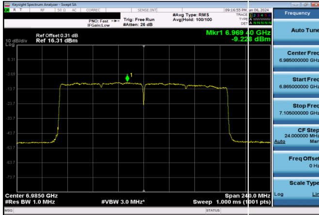
Plot 7-657. Power Spectral Density Plot SDM Diversity Antenna 3b LPI (160MHz 802.11ax (UNII Band 8) – Ch. 207, MCS4)
