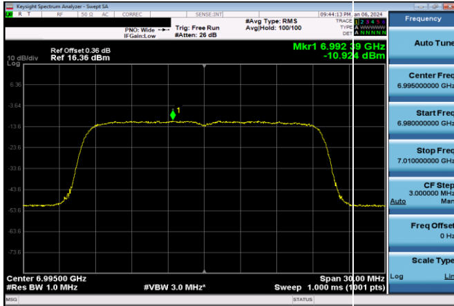
Plot 7-683. Power Spectral Density Plot SDM Diversity Antenna 3b LPI (20MHz 802.11ax (UNII Band 8) – Ch. 209, MCS11)
