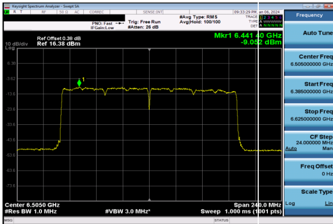
Plot 7-673. Power Spectral Density Plot SDM Diversity Antenna 3b LPI (160MHz 802.11ax (UNII Band 6) – Ch. 111, MCS11)
