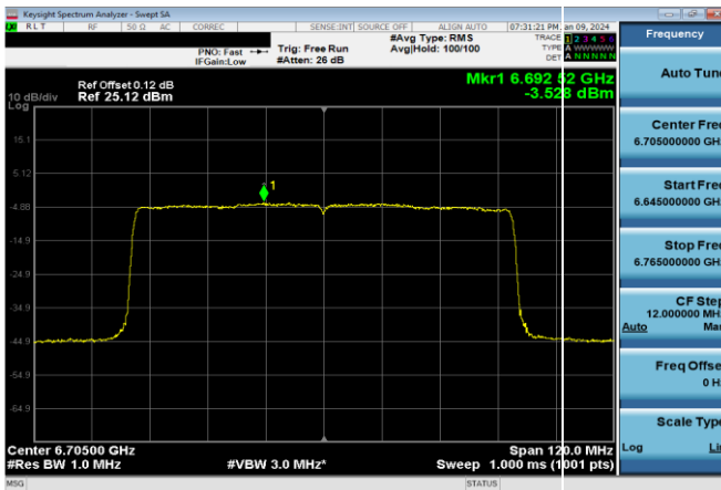
Plot 7-704. Power Spectral Density Plot CDD Diversity Antenna 1b Standard Power (80MHz 802.11ax (UNII Band 7) – Ch. 151, MCS2)
