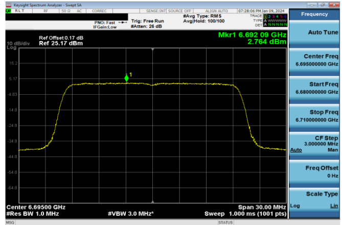
Plot 7-700. Power Spectral Density Plot CDD Diversity Antenna 1b Standard Power (20MHz 802.11ax (UNII Band 7) – Ch. 149, MCS2)
