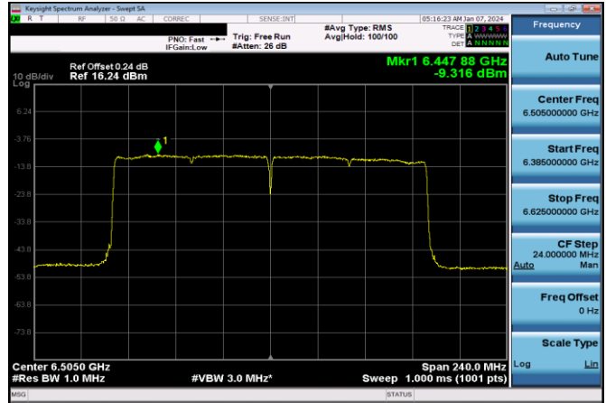
Plot 7-610. Power Spectral Density Plot SDM Diversity Antenna 1b LPI (160MHz 802.11ax (UNII Band 6) – Ch. 111, MCS2)
