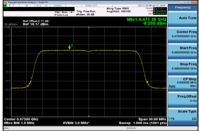
Plot 7-604. Power Spectral Density Plot SDM Diversity Antenna 1b LPI (20MHz 802.11ax (UNII Band 6) – Ch. 105, MCS2)
