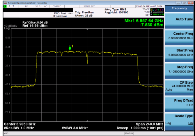
Plot 7-420. Power Spectral Density Plot Antenna 1b LPI (160MHz 802.11ax (UNII Band 8) – Ch. 207, MCS11)
