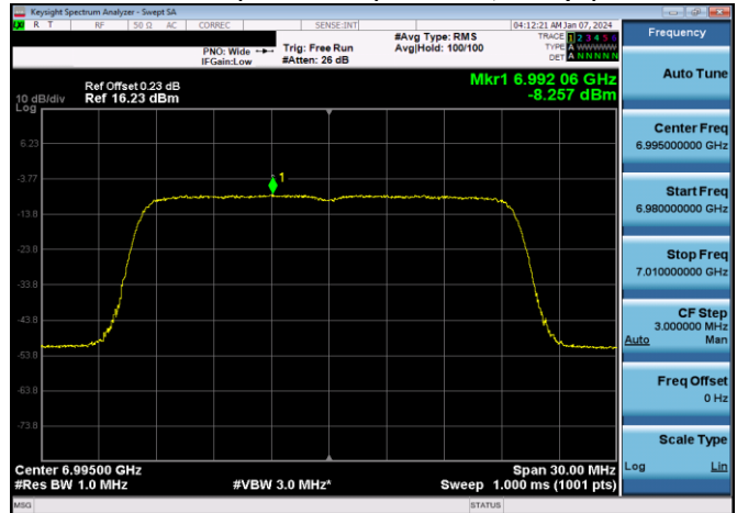
Plot 7-397. Power Spectral Density Plot Antenna 1b LPI (20MHz 802.11ax (UNII Band 8) – Ch. 209, MCS4)
