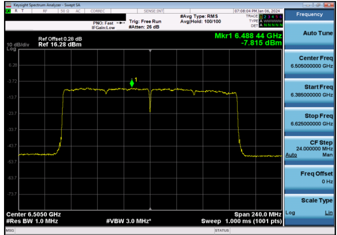
Plot 7-300. Power Spectral Density Plot Antenna 3b LPI (160MHz 802.11ax (UNII Band 6) – Ch. 111, MCS4)
