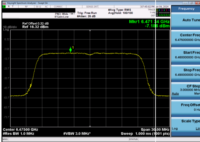
Plot 7-317. Power Spectral Density Plot Antenna 3b LPI (20MHz 802.11ax (UNII Band 6) – Ch. 105, MCS11)
