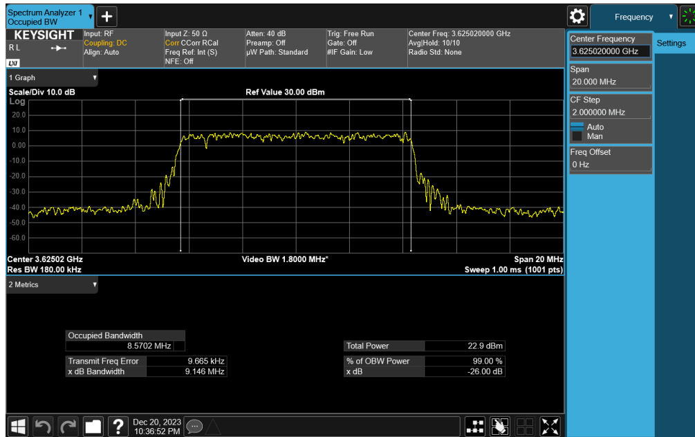
Plot 7-33. Occupied Bandwidth Plot (NR Band n48 - 10MHz DFT-s-OFDM \pi/2 BPSK - Full RB Configuration)
