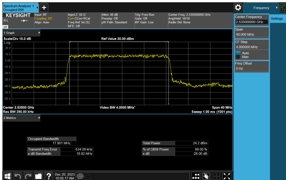
Plot 7-66. Occupied Bandwidth Plot (NR Band n7 - 20MHz DFT-s-OFDM \pi/2 BPSK - Full RB)
