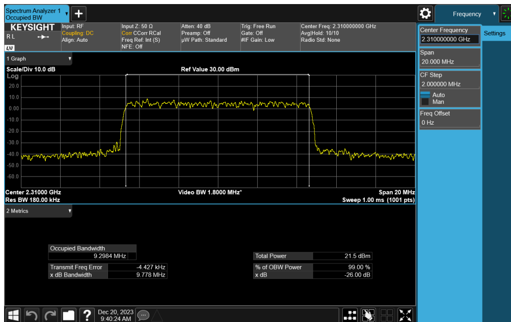
Plot 7-48. Occupied Bandwidth Plot (NR Band n30 - 10MHz CP-OFDM 16-QAM - Full RB)
