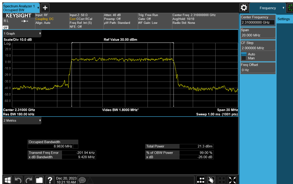
Plot 7-46. Occupied Bandwidth Plot (NR Band n30 - 10MHz DFT-s-OFDM \pi/2 BPSK - Full RB)
