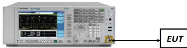
Figure 7-3. Test Instrument & Measurement Setup
