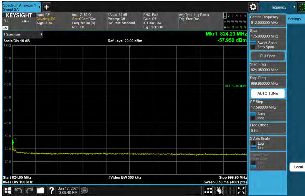
Plot 7-76. Conducted Spurious Plot (NR Band 26 - 10MHz DFT-s-OFDM QPSK - RB Size 1, RB Offset 0 - Mid Channel)
