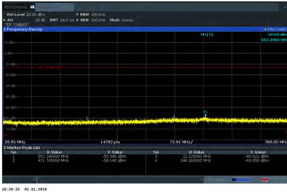
Plot 7-60. Conducted Spurious Plot (LTE Band 14 - 5MHz QPSK - RB Size 1, RB Offset 0 - High Channel)
