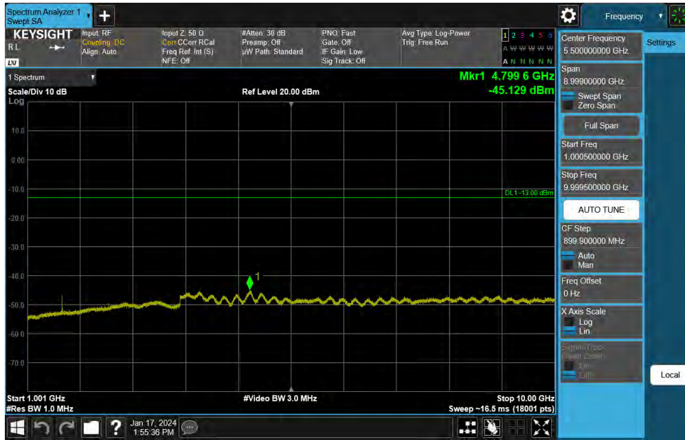
Plot 7-71. Conducted Spurious Plot (NR Band 14 - 5MHz DFT-s-OFDM QPSK - RB Size 1, RB Offset 0 - High Channel)
