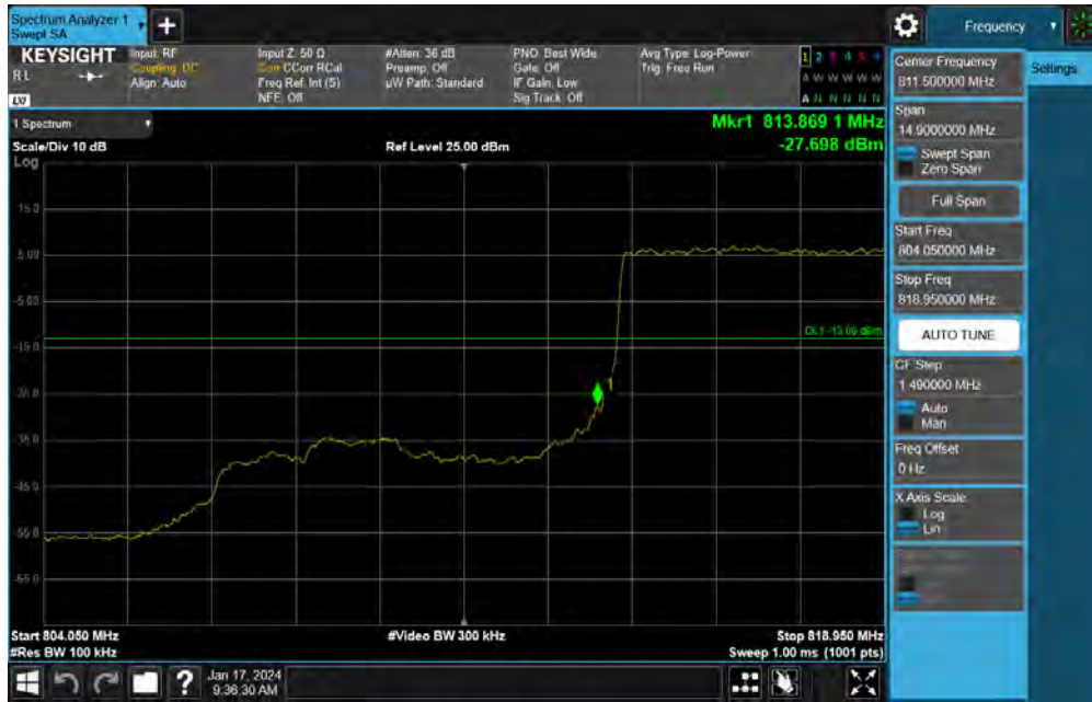
Plot 7-107. Lower Band Edge Plot (NR Band n26 - 10MHz DFT-s-OFDM \pi/2 BPSK – Low Channel)
