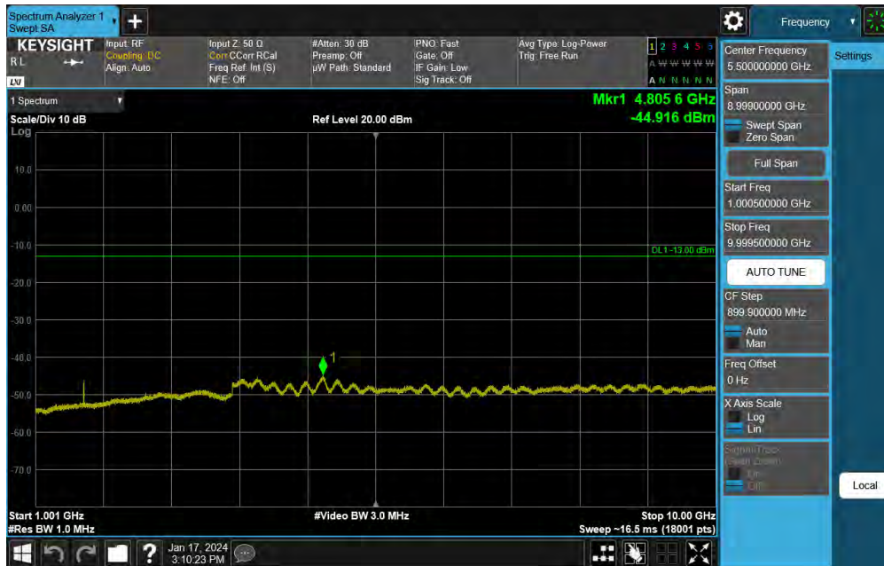
Plot 7-77. Conducted Spurious Plot (NR Band 26 - 10MHz DFT-s-OFDM QPSK - RB Size 1, RB Offset 0 - Mid Channel)
