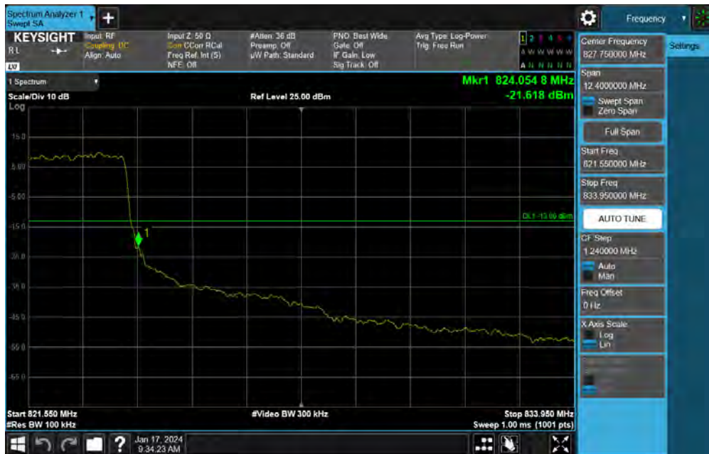
Plot 7-106. Upper Band Edge Plot (NR Band n26 - 5MHz DFT-s-OFDM QPSK – High Channel)
