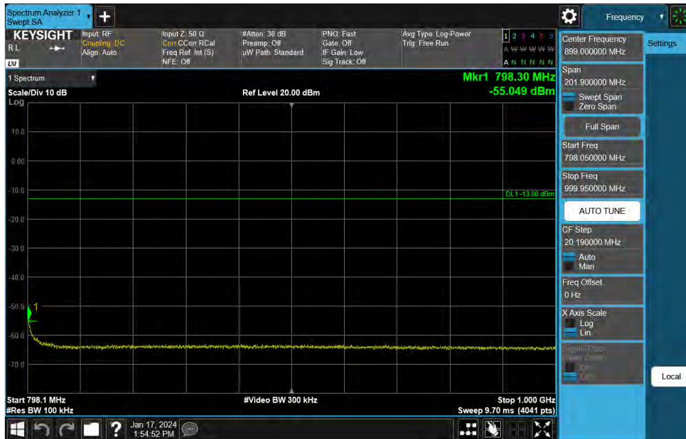
Plot 7-70. Conducted Spurious Plot (NR Band 14 - 5MHz DFT-s-OFDM QPSK - RB Size 1, RB Offset 0 - High Channel)
