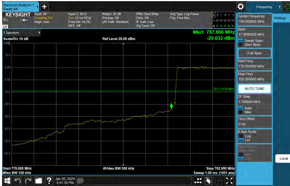
Plot 7-101. Lower Band Edge Plot (NR Band n14 - 10MHz QPSK – RB Size 50)
