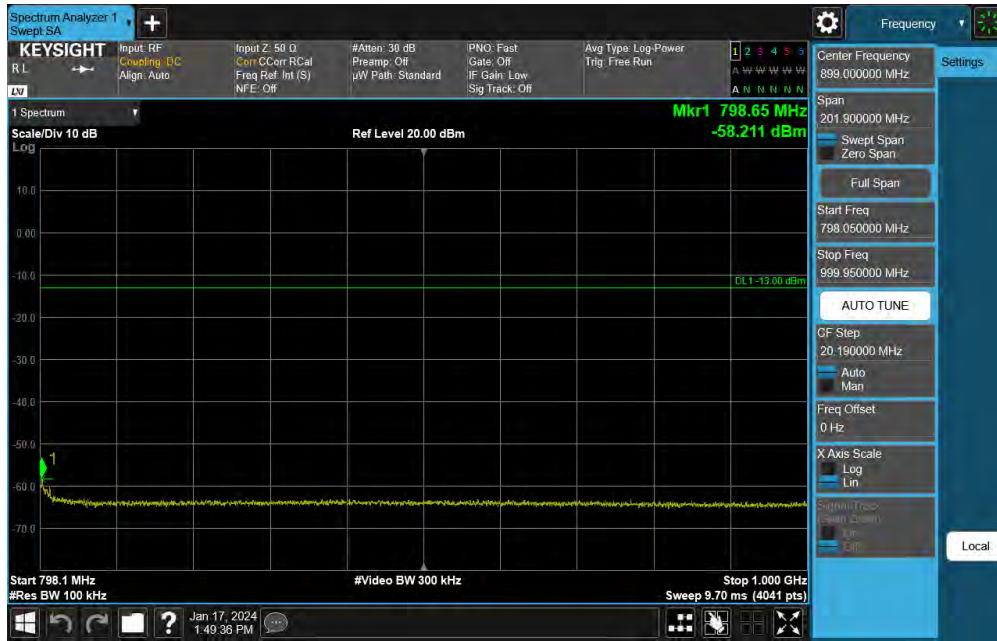
Plot 7-67. Conducted Spurious Plot (NR Band 14 - 10MHz DFT-s-OFDM QPSK - RB Size 1, RB Offset 0 - Mid Channel)
