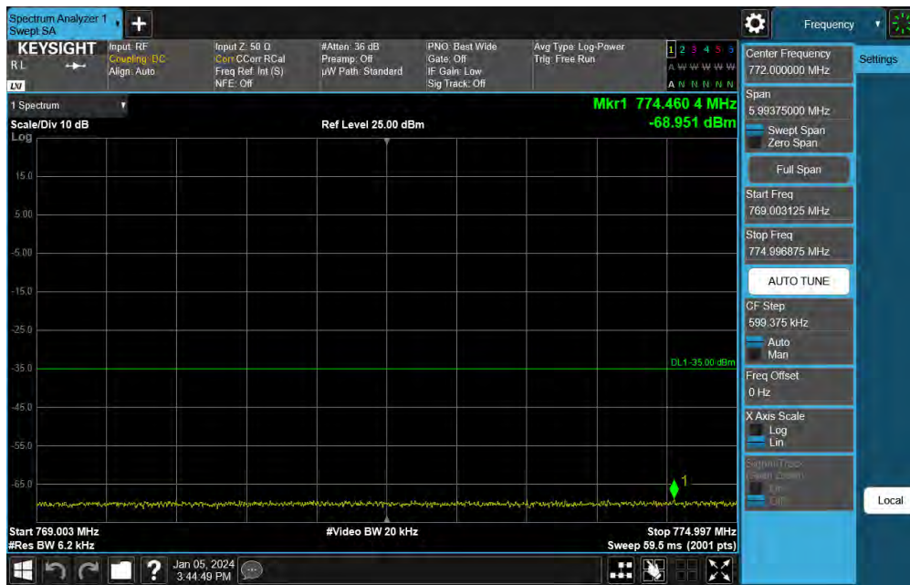
Plot 7-102. Lower Emission Mask Plot (NR Band n14 - 10MHz DFT-s-OFDM \pi/2 BPSK – RB Size 50)
