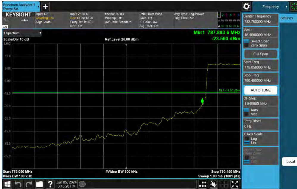
Plot 7-97. Lower Band Edge Plot (NR Band n14 - 5MHz DFT-s-OFDM \pi/2 BPSK – RB Size 25)
