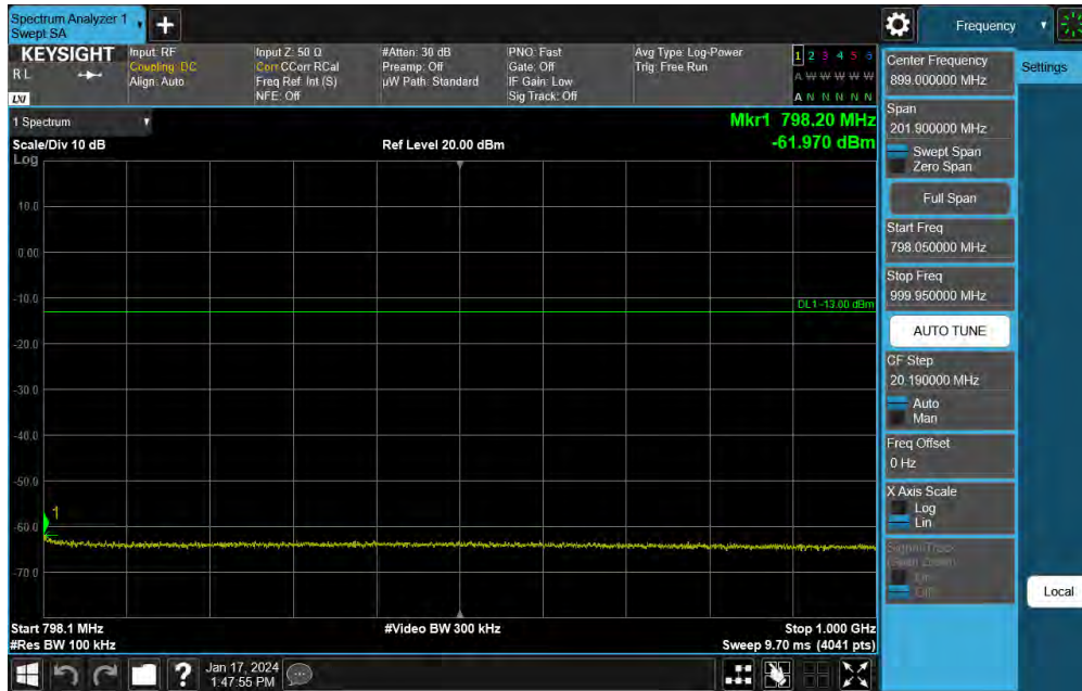
Plot 7-64. Conducted Spurious Plot (NR Band 14 - 5MHz DFT-s-OFDM QPSK - RB Size 1, RB Offset 0 - Low Channel)
