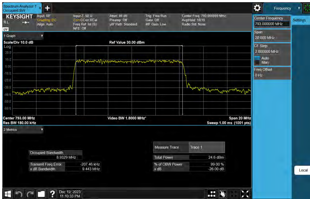
Plot 7-30. Occupied Bandwidth Plot (NR Band 14 - 10MHz DFT-s-OFDM \pi/2 BPSK - Full RB)
