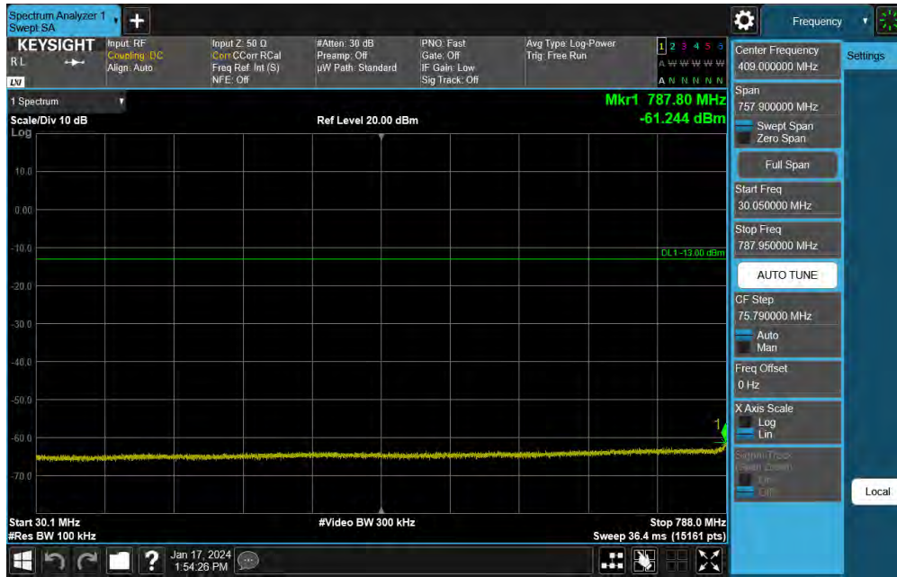
Plot 7-69. Conducted Spurious Plot (NR Band 14 - 5MHz DFT-s-OFDM QPSK - RB Size 1, RB Offset 0 - High Channel)
