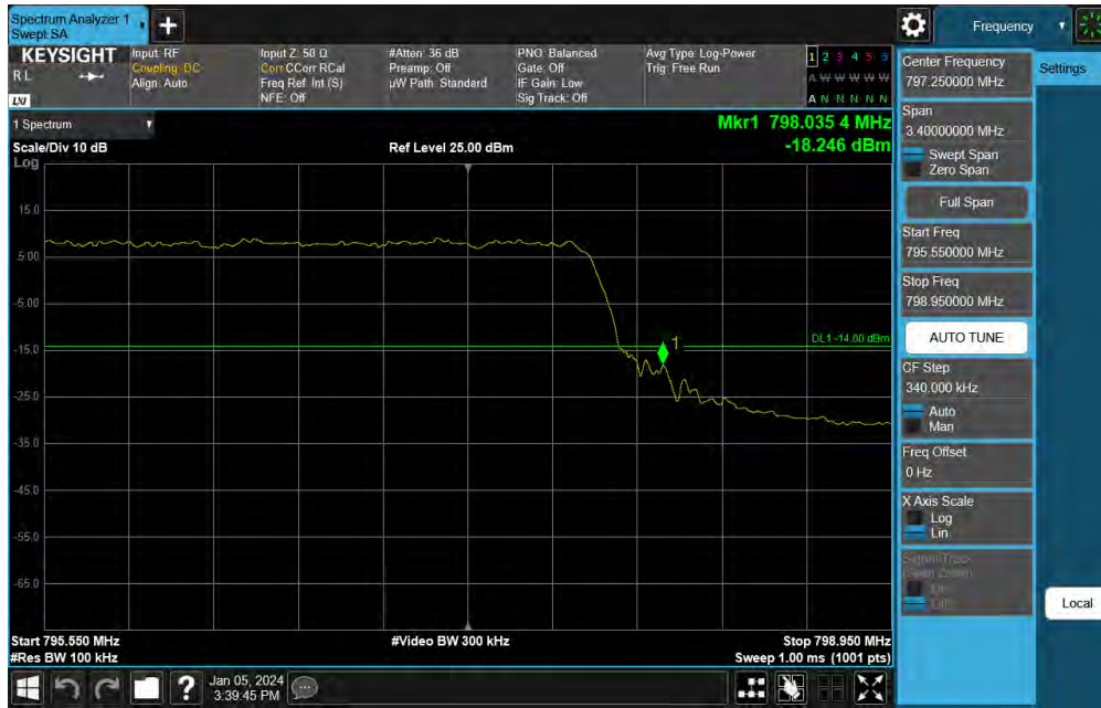
Plot 7-99. Upper Band Edge Plot (NR Band n14 - 5MHz DFT-s-OFDM QPSK – RB Size 25)
