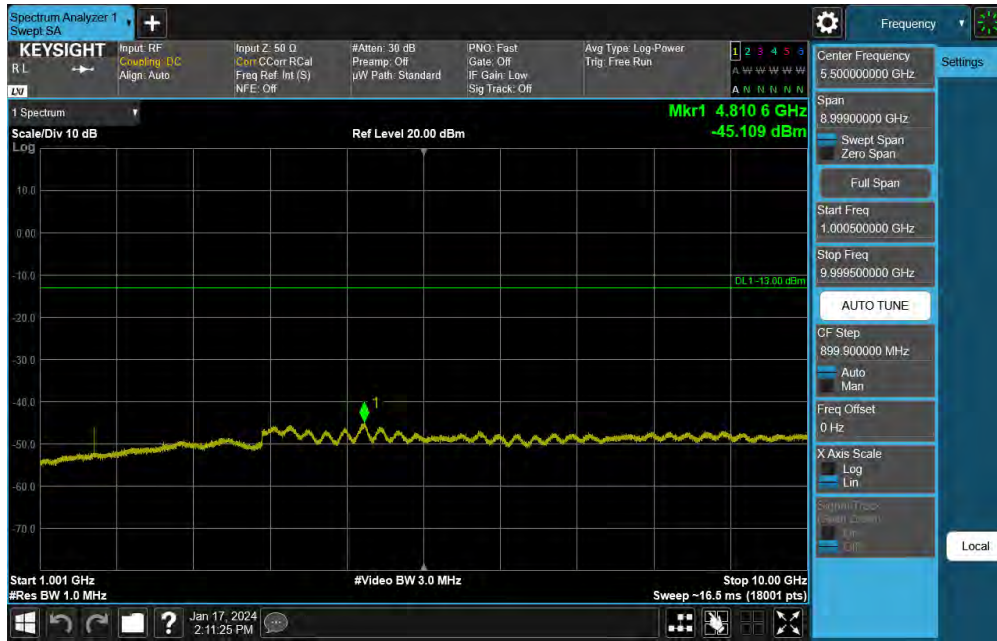
Plot 7-74. Conducted Spurious Plot (NR Band 26 - 5MHz DFT-s-OFDM QPSK - RB Size 1, RB Offset 0 - Low Channel)
