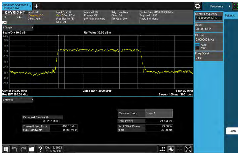
Plot 7-40. Occupied Bandwidth Plot (NR Band 26 - 10MHz DFT-s-OFDM \pi/2 BPSK - Full RB)
