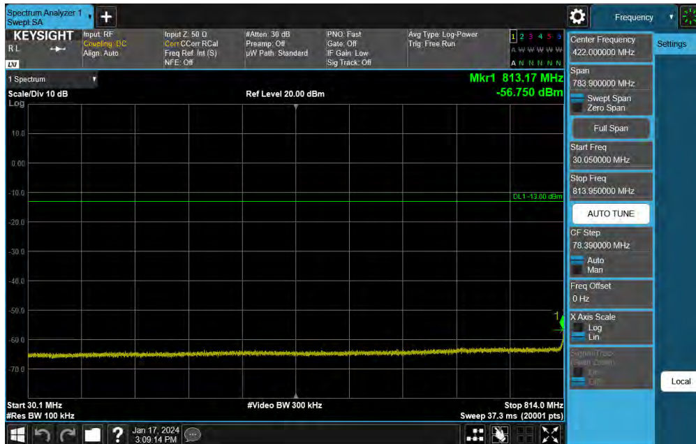
Plot 7-75. Conducted Spurious Plot (NR Band 26 - 10MHz DFT-s-OFDM QPSK - RB Size 1, RB Offset 0 - Mid Channel)
