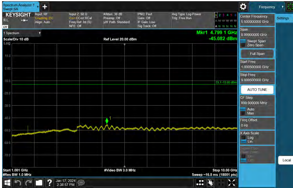
Plot 7-80. Conducted Spurious Plot (NR Band 26 - 5MHz DFT-s-OFDM QPSK - RB Size 1, RB Offset 0 - High Channel)
