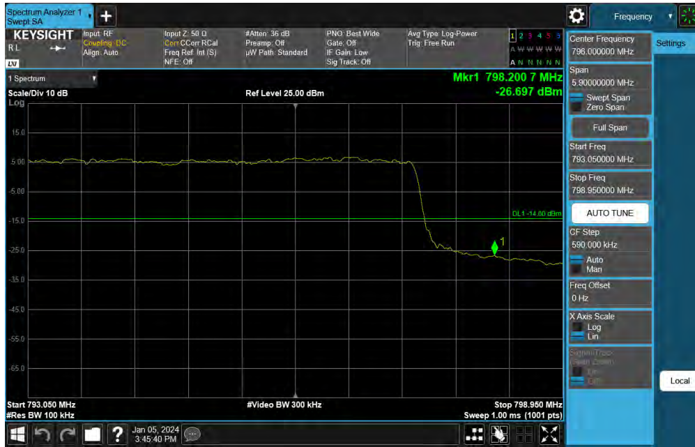
Plot 7-103. Upper Band Edge Plot (NR Band n14 - 10MHz DFT-s-OFDM \pi/2 BPSK – RB Size 50)
