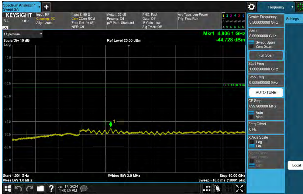
Plot 7-65. Conducted Spurious Plot (NR Band 14 - 5MHz DFT-s-OFDM QPSK - RB Size 1, RB Offset 0 - Low Channel)
