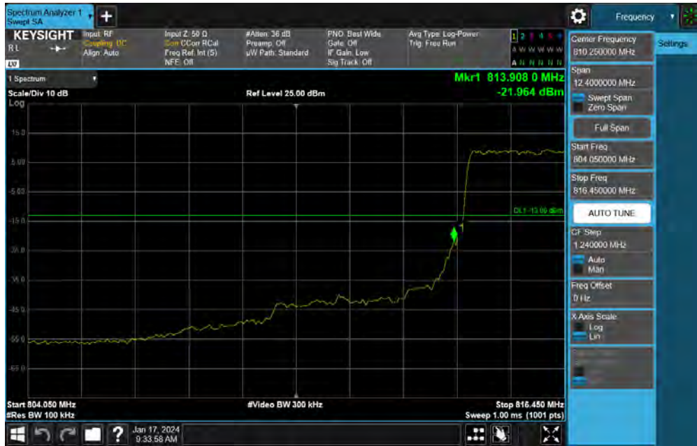
Plot 7-105. Lower Band Edge Plot (NR Band n26 - 5MHz DFT-s-OFDM QPSK – Low Channel)
