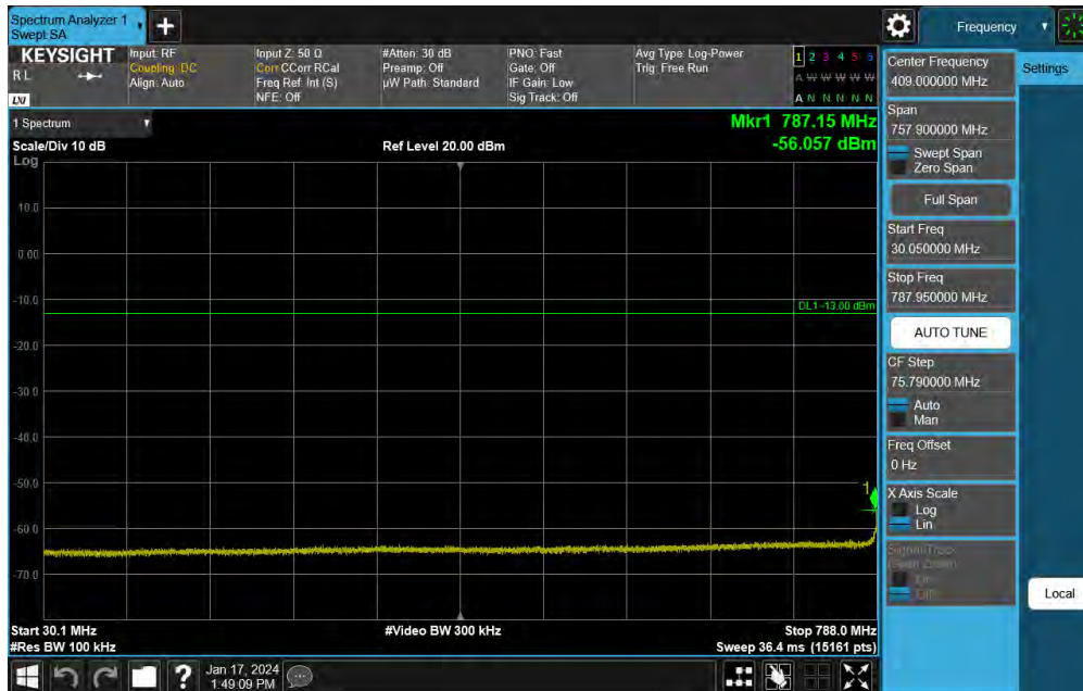
Plot 7-66. Conducted Spurious Plot (NR Band 14 - 10MHz DFT-s-OFDM QPSK - RB Size 1, RB Offset 0 - Mid Channel)
