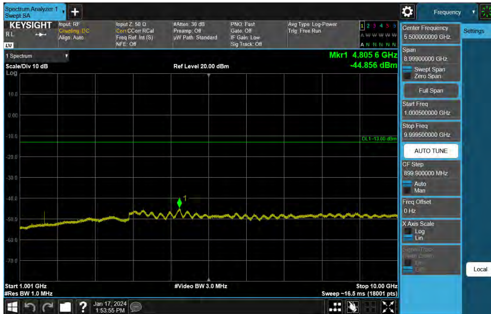
Plot 7-68. Conducted Spurious Plot (NR Band 14 - 10MHz DFT-s-OFDM QPSK - RB Size 1, RB Offset 0 - Mid Channel)
