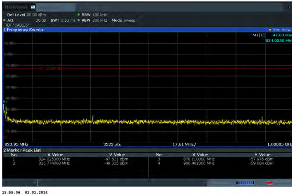
Plot 7-52. Conducted Spurious Plot (LTE Band 26 - 5MHz QPSK - RB Size 1, RB Offset 0 - High Channel)
