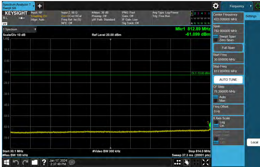
Plot 7-78. Conducted Spurious Plot (NR Band 26 - 5MHz DFT-s-OFDM QPSK - RB Size 1, RB Offset 0 - High Channel)
