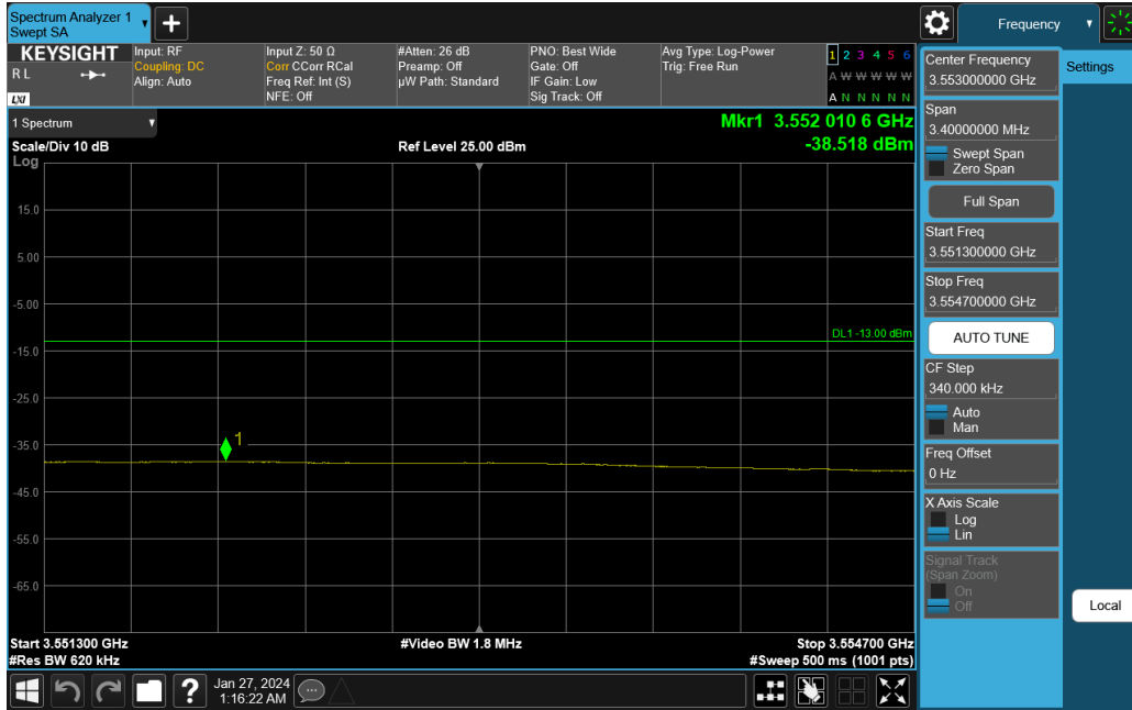
Plot 7-183. Upper ACP Plot (NR Band n77 DoD-Band - 60MHz DFT-s-OFDM QPSK – Full RB)
