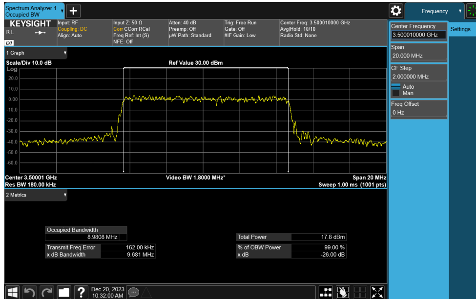
Plot 7-5. Occupied Bandwidth Plot (NR Band n77 DoD-Band - 10MHz CP-OFDM 256-QAM - Full RB)
