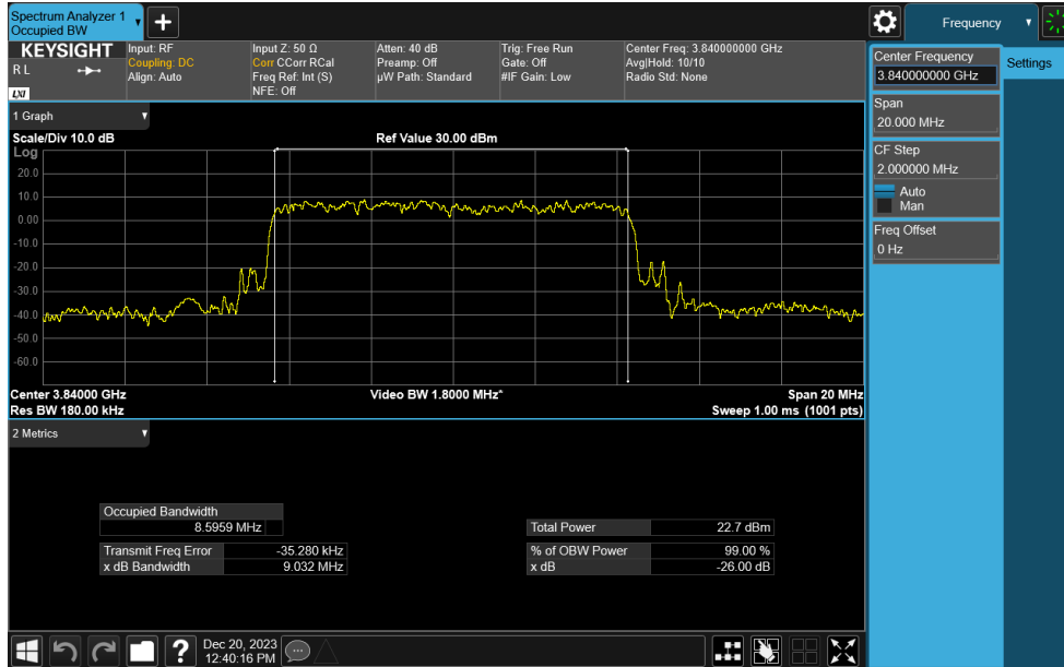
Plot 7-56. Occupied Bandwidth Plot (NR Band n77 C-Band - 10MHz DFT-s-OFDM \pi/2 BPSK - Full RB)
