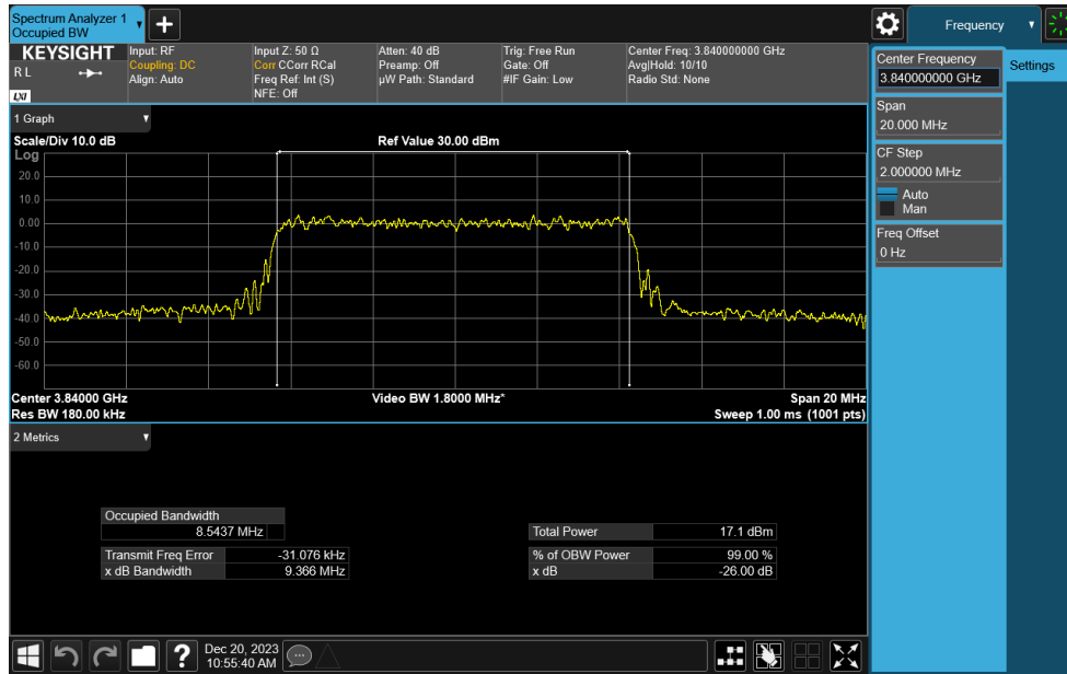
Plot 7-60. Occupied Bandwidth Plot (NR Band n77 C-Band - 10MHz CP-OFDM 256-QAM - Full RB)
