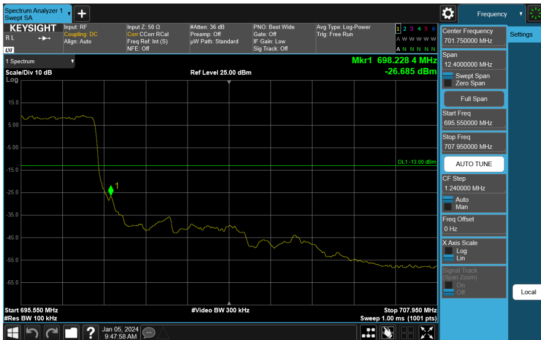
Plot 7-357. Upper Band Edge Plot (NR Band n71 – 5.0MHz DFT-s-OFDM \pi/2 BPSK - Full RB)
