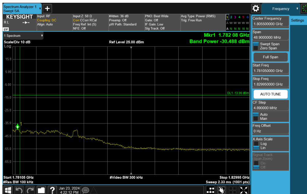
Plot 7-339. Upper Extended Band Edge Plot (NR Band n66 – 35.0MHz DFT-s-OFDM \pi/2 BPSK - Full RB)
