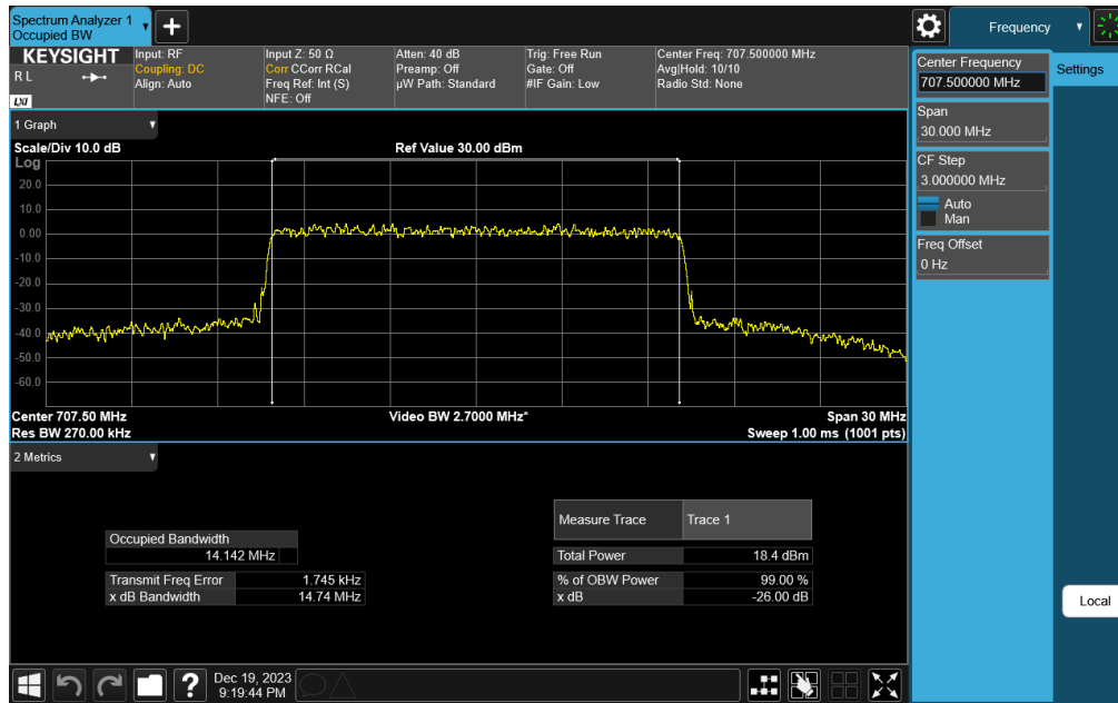
Plot 7-154. Occupied Bandwidth Plot (NR Band n12 - 15MHz CP-OFDM 256-QAM - Full RB)
