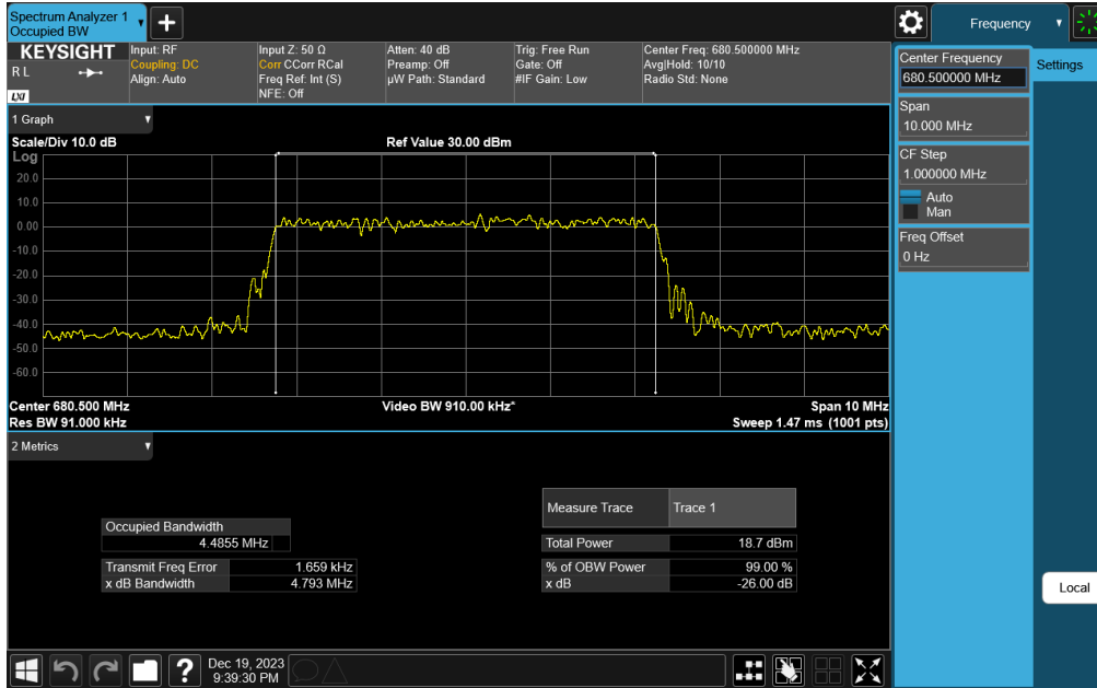
Plot 7-124. Occupied Bandwidth Plot (NR Band n71 - 5MHz CP-OFDM 256-QAM - Full RB)
