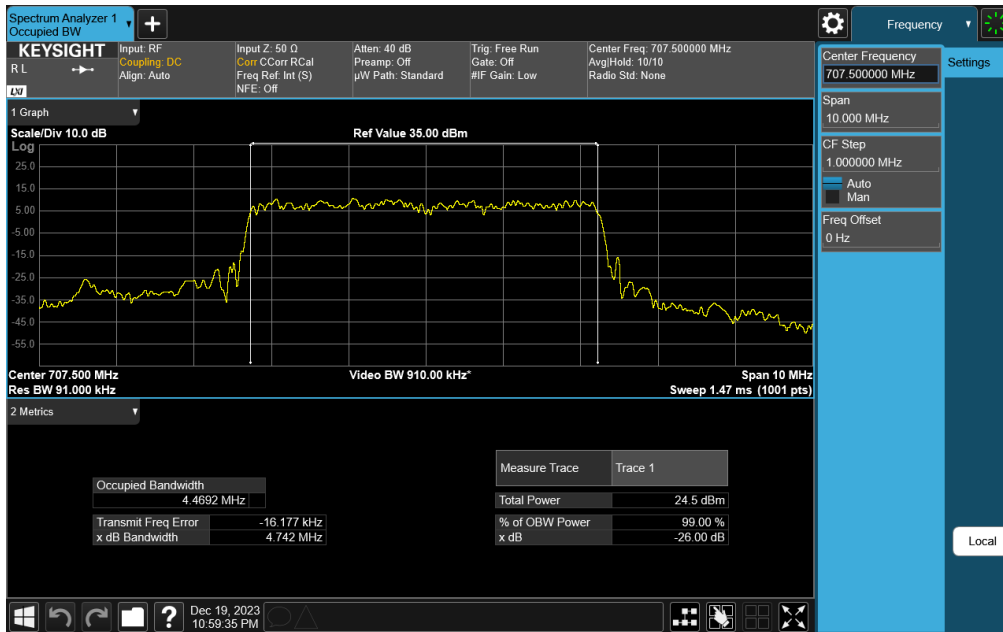
Plot 7-140. Occupied Bandwidth Plot (NR Band n12 - 5MHz DFT-s-OFDM \pi/2 BPSK - Full RB)
