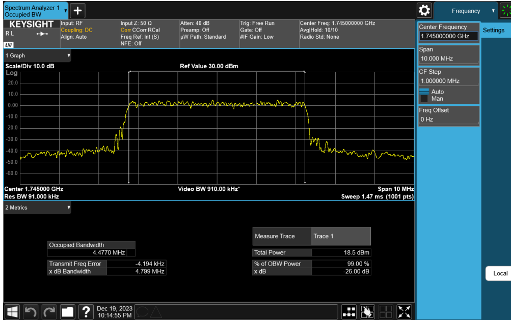
Plot 7-69. Occupied Bandwidth Plot (NR Band n66 - 5.0MHz CP-OFDM 256QAM - Full RB)
