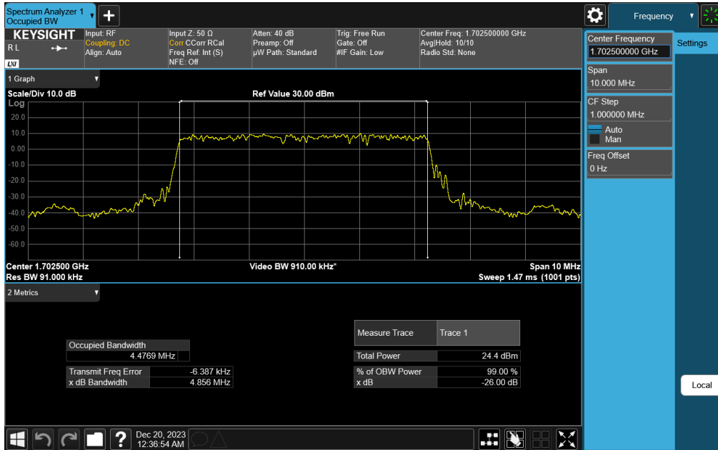
Plot 7-105. Occupied Bandwidth Plot (NR Band n70 - 5MHz DFT-s-OFDM \pi/2 BPSK - Full RB)
