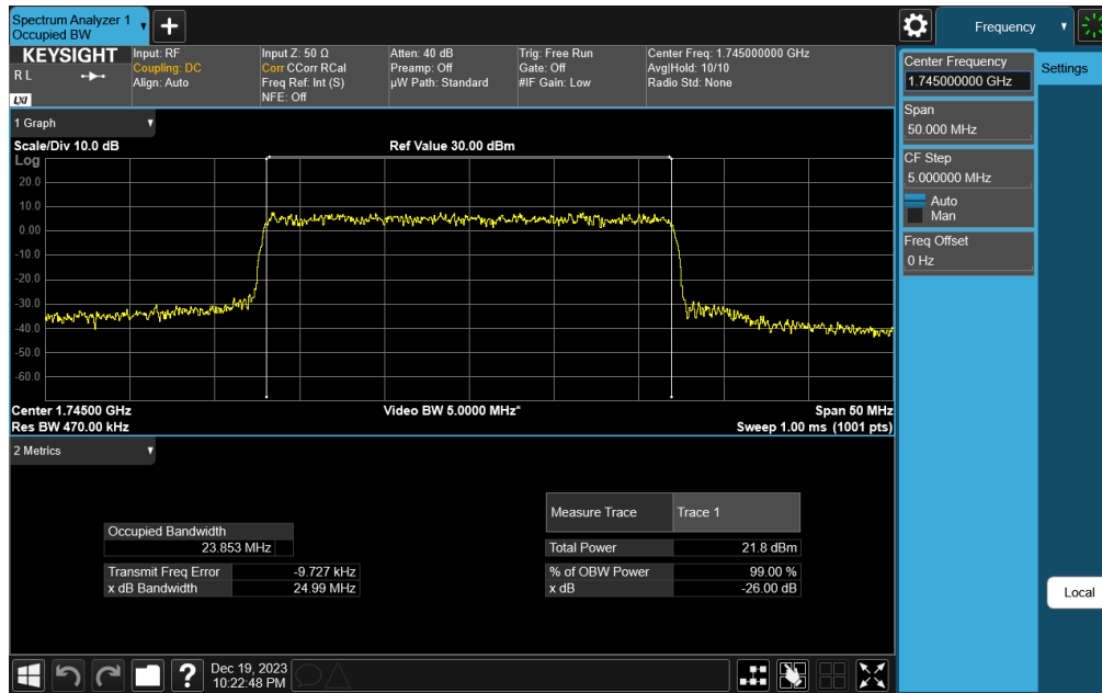
Plot 7-87. Occupied Bandwidth Plot (NR Band n66 - 25.0MHz CP-OFDM 16QAM - Full RB)
