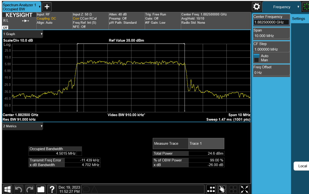
Plot 7-25. Occupied Bandwidth Plot (NR Band n25/n2 - 5MHz DFT-s-OFDM \pi/2 BPSK - Full RB)
