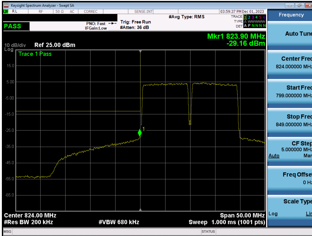
Plot 7-94. Lower BE Plot (ULCA – LTE Band 5 – (10 + 10)MHz QPSK – Full RB Configuration)
