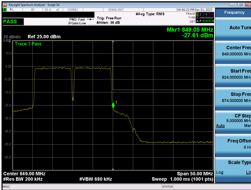
Plot 7-95. Upper BE Plot (ULCA – LTE Band 5 - (10 + 10)MHz QPSK – Full RB Configuration)
