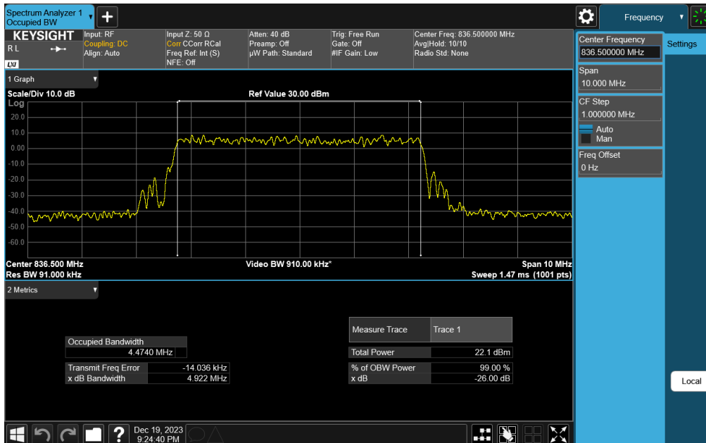
Plot 7-22. Occupied Bandwidth Plot (NR Band n26/n5 - 5MHz CP-OFDM QPSK - Full RB Configuration)
