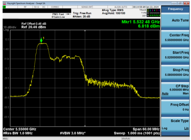
Plot 7-588. PSD CDD Diversity Antenna 5T (40MHz BW 11ax Index 37 - RU52 - Ch.110)
