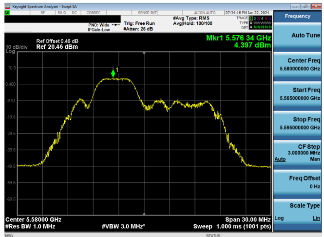
Plot 7-583. PSD CDD Diversity Antenna 1b (20MHz BW 11ax Index 38 – RU52 – Ch.116)
