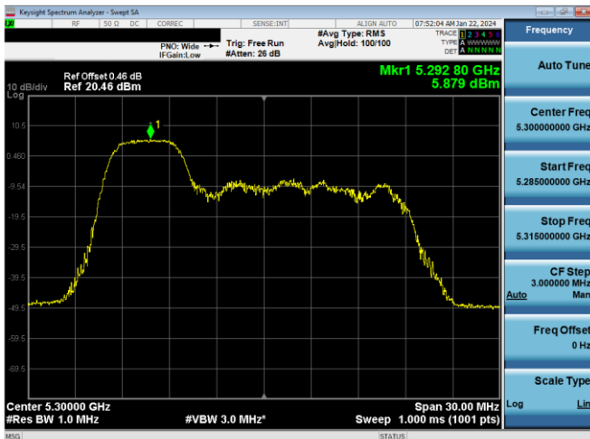
Plot 7-556. PSD CDD Diversity Antenna 5T (20MHz BW 11ax Index 37 – RU52 – Ch.60)
