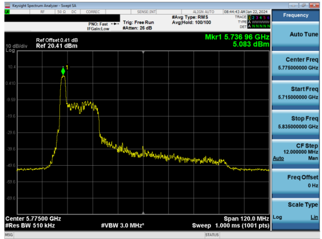
Plot 7-486. PSD CDD Primary Antenna 5T (80MHz BW 11ax Index 0 - RU26 - Ch.155)
