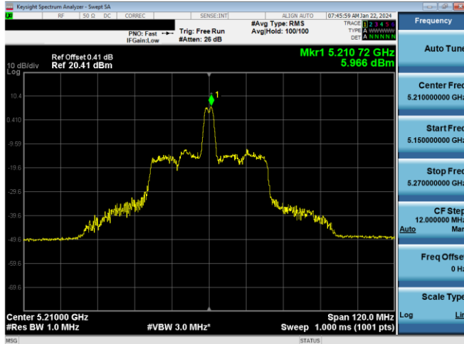
Plot 7-542. PSD CDD Diversity Antenna 5T (80MHz BW 11ax Index 18 - RU26 - Ch.42)
