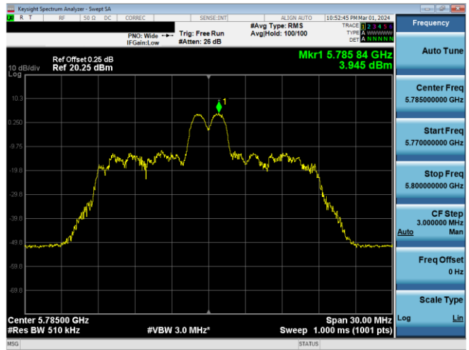
Plot 7-473. PSD CDD Primary Antenna 3b (20MHz BW 11ax Index 4 – RU26 – Ch.157)
