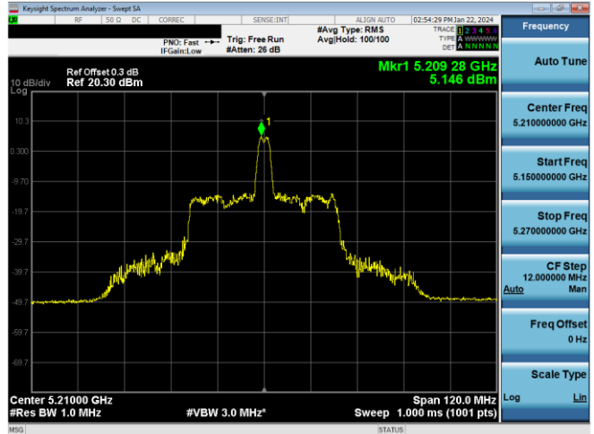
Plot 7-320. PSD Antenna 1b (80MHz BW 11ax Index 18 - RU26 - Ch.42)
