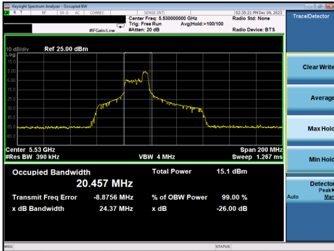
Plot 7-126. 26dB BW & 99% OBW Antenna 1b (80MHz BW 11ax Index 44 – RU52 – Ch.106)
