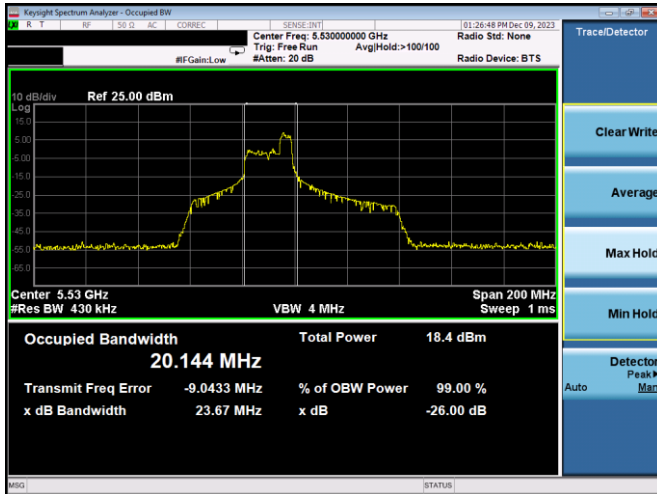
Plot 7-82. 26dB BW & 99% OBW Antenna 3b (80MHz BW 11ax Index 44 – RU52 – Ch.106)
