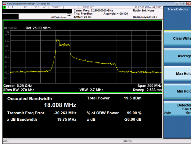
Plot 7-25. 26dB BW & 99% OBW Antenna 5T (80MHz BW 11ax Index 37 – RU52 – Ch.58)
