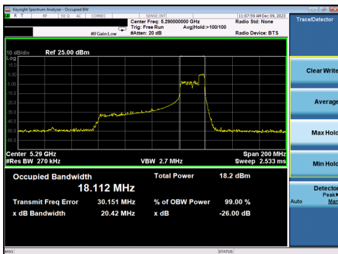
Plot 7-27. 26dB BW & 99% OBW Antenna 5T (80MHz BW 11ax Index 52 – RU52 – Ch.58)
