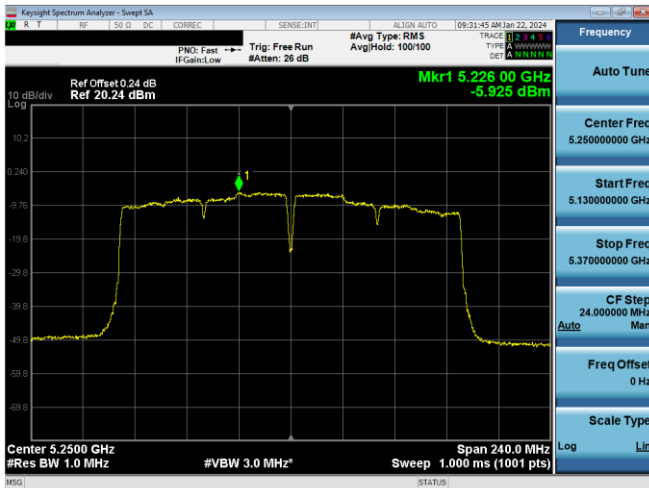
Plot 7-591. PSD CDD Primary Antenna 5T (160MHz BW 802.11ac - Ch. 50, MCS2)
