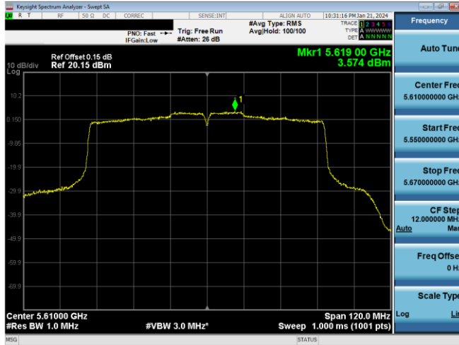
Plot 7-271. PSD Antenna 5T (80MHz BW 802.11ac – Ch. 122, MCS2)
