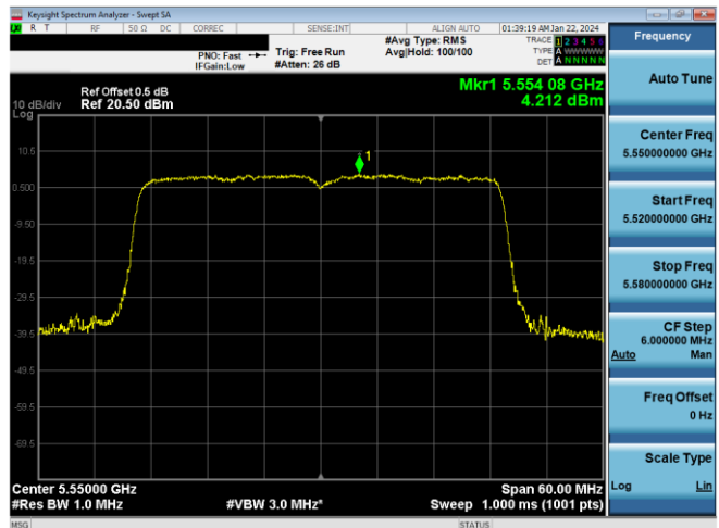
Plot 7-314. PSD Antenna 5T (40MHz BW 802.11ax(SU) – Ch. 110, MCS11)
