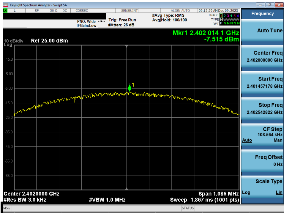
Plot 7-44. Power Spectral Density Plot Antenna 1a (Bluetooth (LE), 1Mbps, iPA – Ch. 0)
