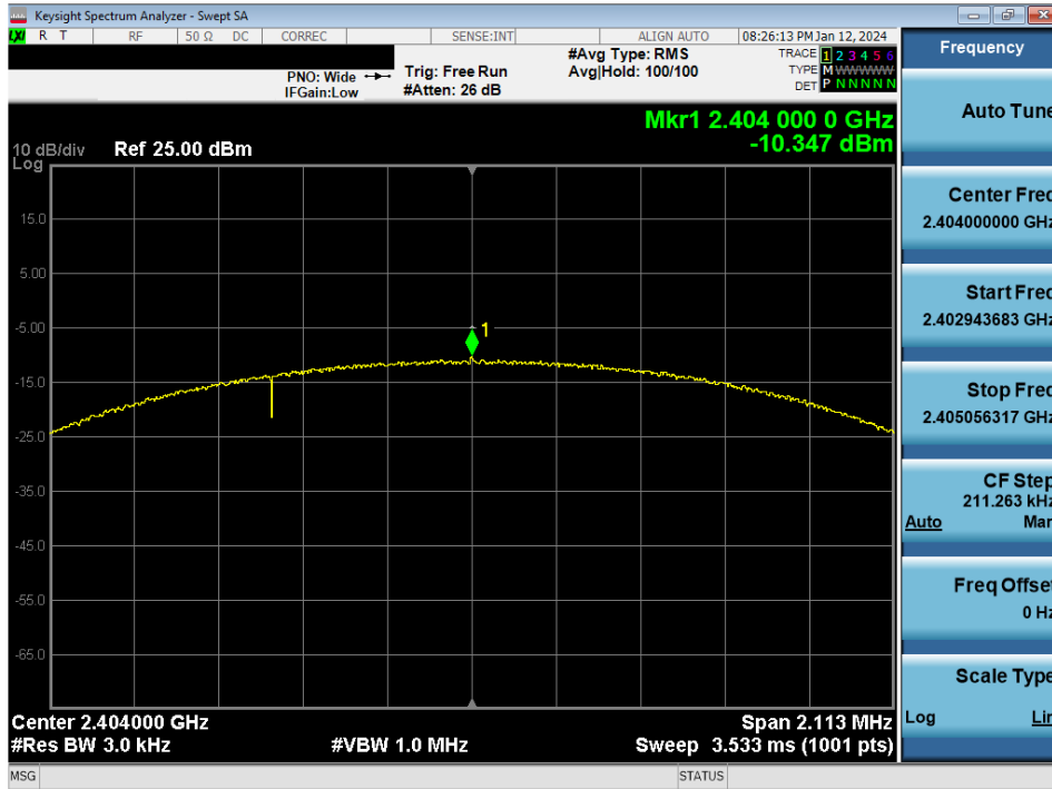
Plot 7-49. Power Spectral Density Plot Antenna 3a (Bluetooth (LE), 2Mbps, ePA – Ch. 1)
