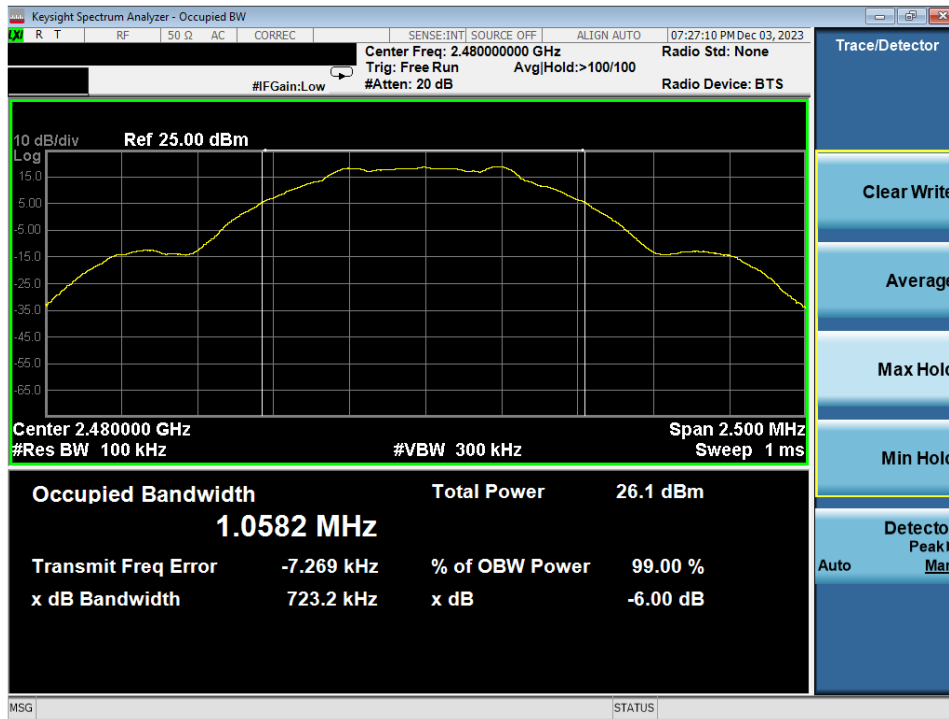
Plot 7-3. 6dB BW & 99% OBW Plot Antenna 3a (Bluetooth (LE), 1Mbps, ePA – Ch. 39)
