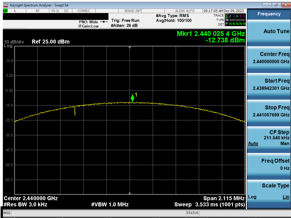
Plot 7-58. Power Spectral Density Plot Antenna 1a (Bluetooth (LE), 2Mbps, iPA – Ch. 19)
