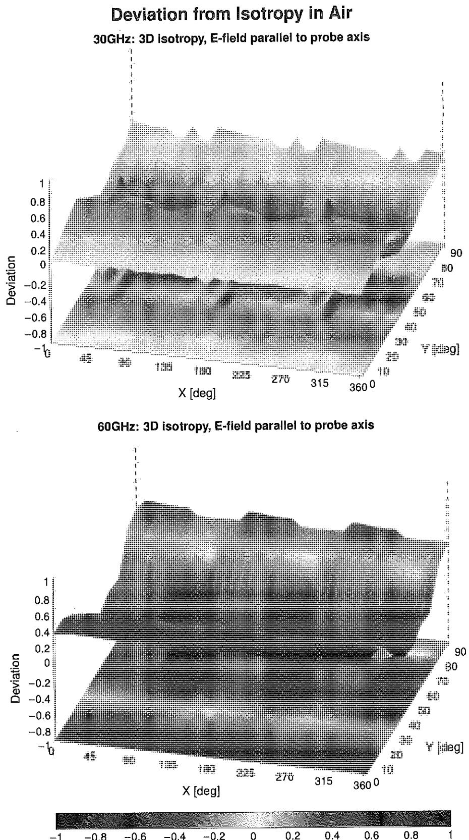
Probe isotropy for  $E_{\text{tot}}$ : probe rotated  $\phi = 0^\circ$  to  $360^\circ$ , tilted from field propagation direction  $\hat{k}$
