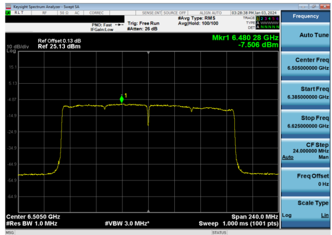
Plot 7-610. Power Spectral Density Plot SDM Diversity Antenna WF7b LPI (160MHz 802.11ax (UNII Band 6) – Ch. 111, MCS2)
