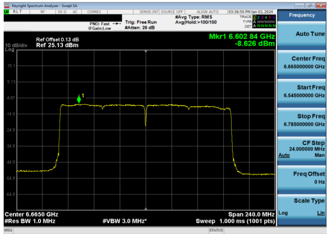
Plot 7-474. Power Spectral Density Plot SDM Primary Antenna WF2a LPI (160MHz 802.11ax (UNII Band 7) – Ch. 143, MCS2)
