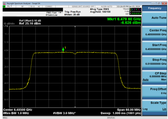
Plot 7-462. Power Spectral Density Plot SDM Primary Antenna WF2a LPI (40MHz 802.11ax (UNII Band 6) – Ch. 107, MCS2)
