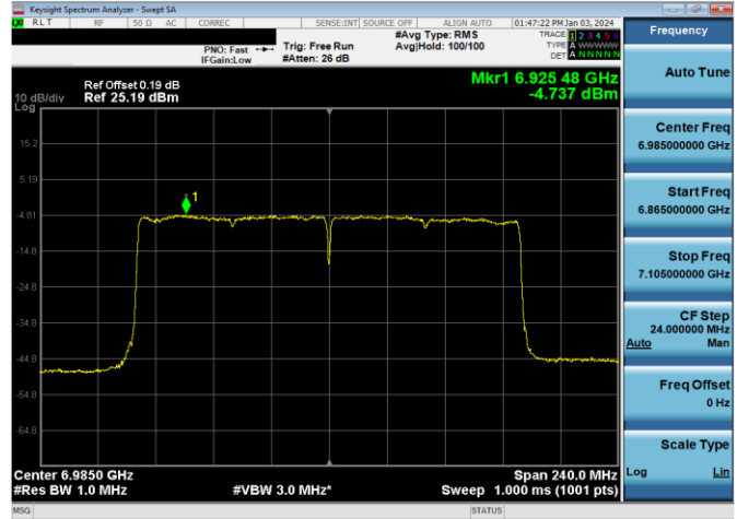
Plot 7-290. Power Spectral Density Plot Antenna WF2a LPI (160MHz 802.11ax (UNII Band 8) – Ch. 207, MCS2)
