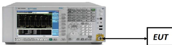
Figure 7-1. Test Instrument & Measurement Setup
