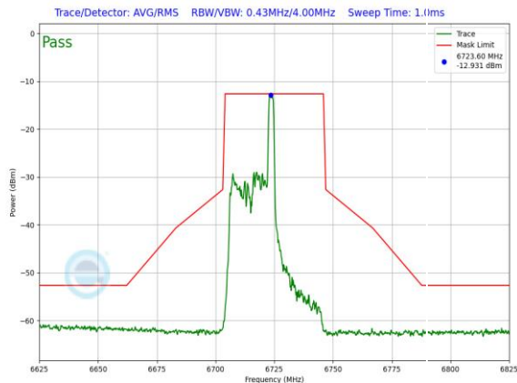
Plot 7-1483. LPI In-Band Emission Plot SDM Diversity Antenna WF7a (40MHz 802.11ax RU26 (UNII Band 7) – Ch. 155)
