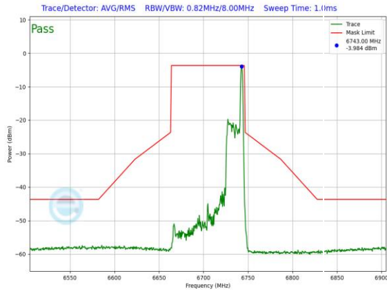
Plot 7-1259. LPI In-Band Emission Plot Antenna WF7b (80MHz 802.11ax RU26 (UNII Band 7) – Ch. 151)
