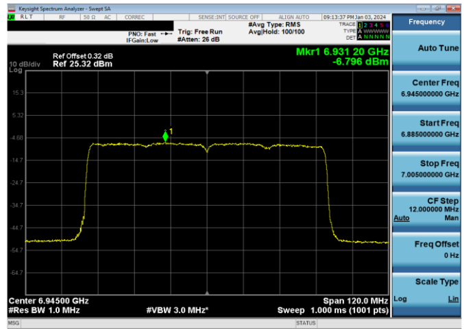
Plot 7-855. LPI Power Spectral Density Plot SDM Antenna WF2a (80MHz 802.11ax RU996 (UNII Band 8) – Ch. 199)
