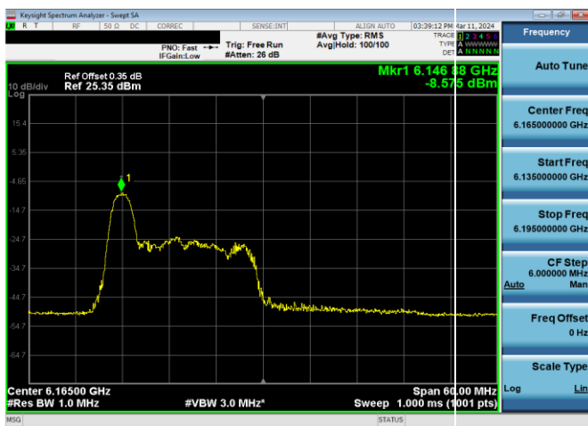
Plot 7-745. LPI Power Spectral Density Plot SDM Antenna WF2a (40MHz 802.11ax RU26 (UNII Band 5) – Ch. 43)
