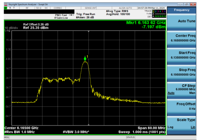
Plot 7-747. LPI Power Spectral Density Plot SDM Antenna WF2a (40MHz 802.11ax RU26 (UNII Band 5) – Ch. 43)
