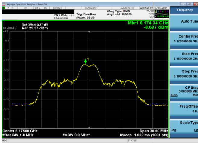
Plot 7-739. LPI Power Spectral Density Plot SDM Antenna WF2a (20MHz 802.11ax RU26 (UNII Band 5) – Ch. 45)
