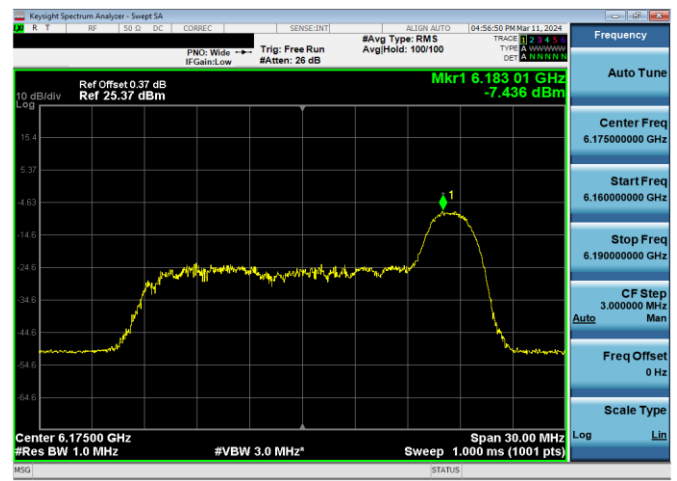
Plot 7-741. LPI Power Spectral Density Plot SDM Antenna WF2a (20MHz 802.11ax RU26 (UNII Band 5) – Ch. 45)
