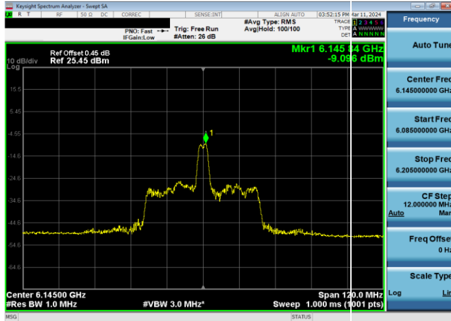
Plot 7-627. LPI Power Spectral Density Plot SDM Antenna WF7a (80MHz 802.11ax RU26 (UNII Band 5) – Ch. 39)
