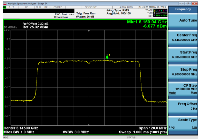
Plot 7-631. LPI Power Spectral Density Plot SDM Antenna WF7a (80MHz 802.11ax RU996 (UNII Band 5) – Ch. 39)
