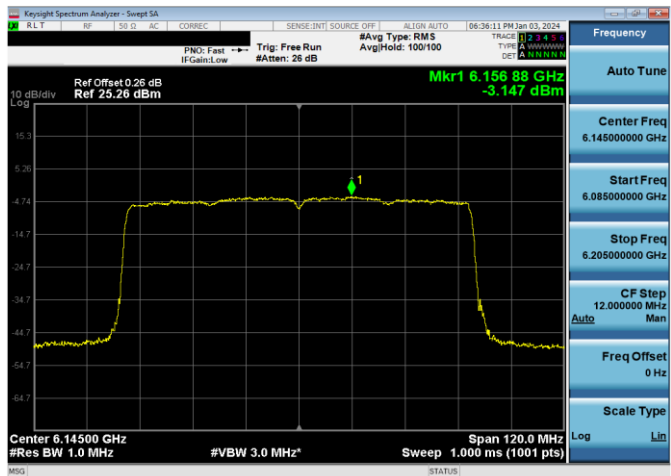
Plot 7-492. LPI Power Spectral Density Plot Antenna WF2a (80MHz 802.11ax RU996 (UNII Band 5) – Ch. 39)
