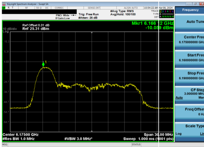
Plot 7-481. LPI Power Spectral Density Plot Antenna WF2a (20MHz 802.11ax RU26 (UNII Band 5) – Ch. 45)
