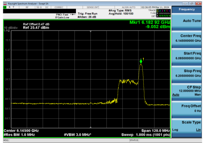
Plot 7-491. LPI Power Spectral Density Plot Antenna WF2a (80MHz 802.11ax RU26 (UNII Band 5) – Ch. 39)
