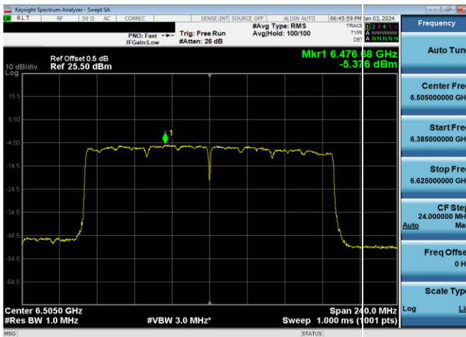
Plot 7-512. LPI Power Spectral Density Plot Antenna WF2a (160MHz 802.11ax RU996x2 (UNII Band 6) – Ch. 111)
