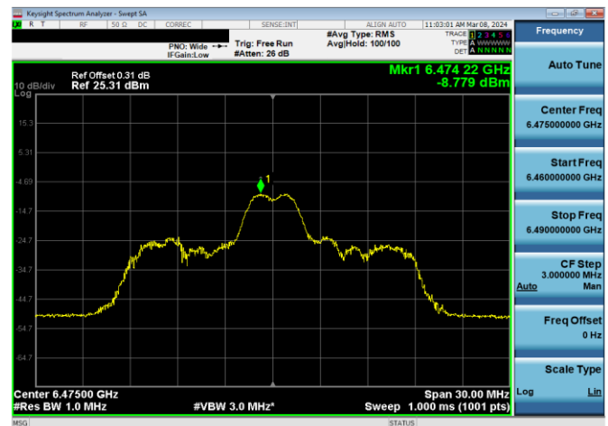
Plot 7-498. LPI Power Spectral Density Plot Antenna WF2a (20MHz 802.11ax RU26 (UNII Band 6) – Ch. 105)
